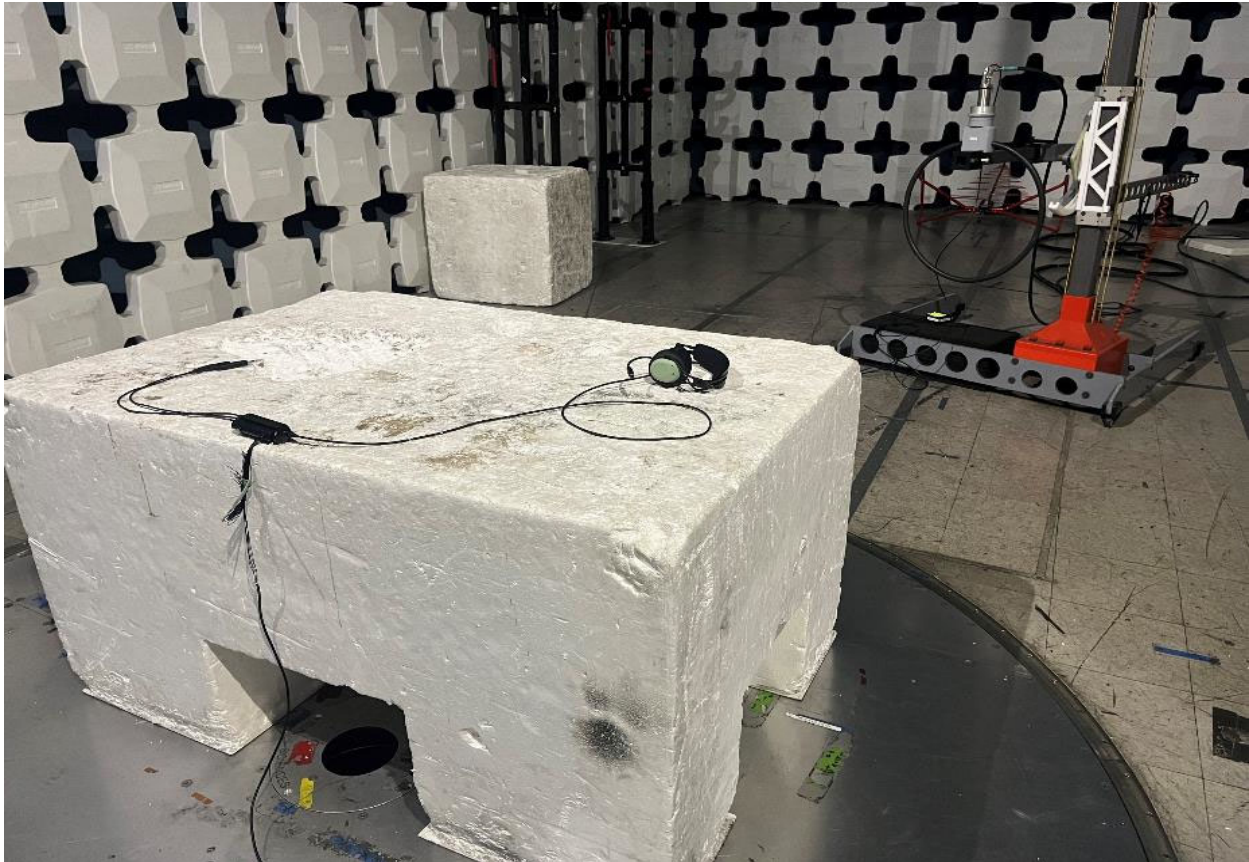
Test Configuration Photograph #1 (Radiated Emissions - Below 30 MHz)
