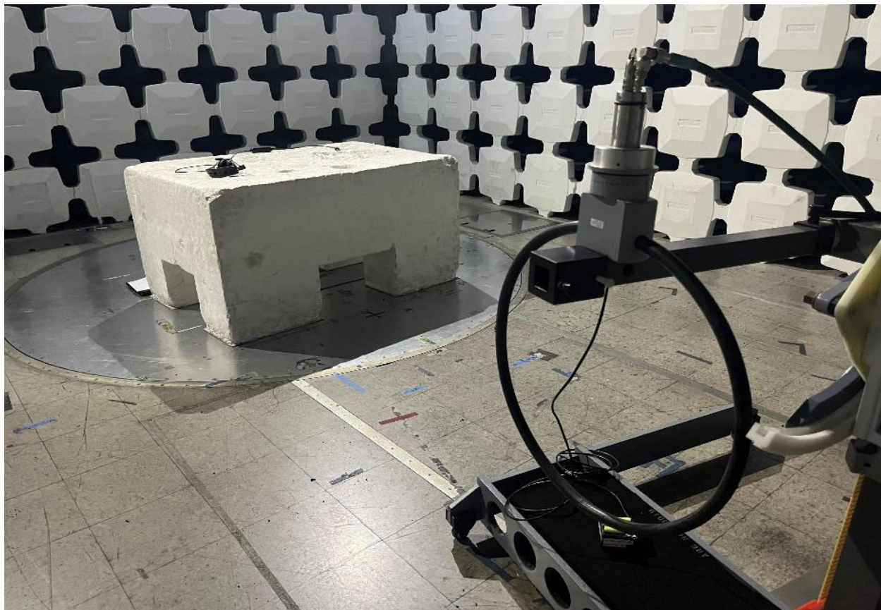
Test Configuration Photograph #3 (Radiated Emissions - Below 30 MHz)
