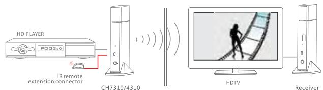
5. When the system working properly, user can use the remote controller of HD player at the HDTV side. the remote controller should be aligned to IR sensor window of transmitter.
