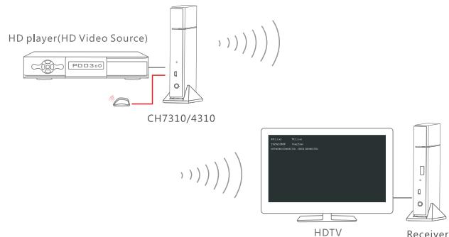
4. wait for the system start, and the screen will display text " Connecting to CH7310." then the images shows up, which means the product is working.
