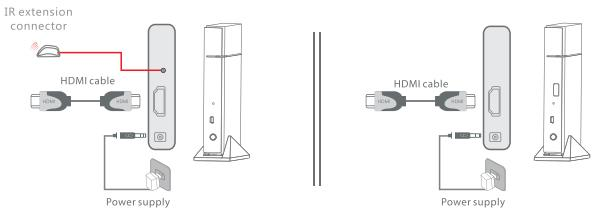
3. Connect the transmitter to the video source device via HDMI cable, then power on the transmitter and video source device. Connect the receiver to the video display device, then turn on the receiver & display device, make sure the network and the video connected properly, the Green light will ON.
