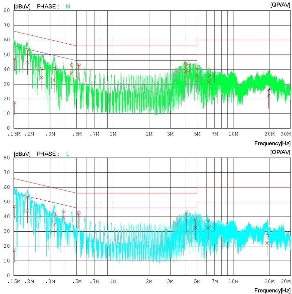
**AC Line Conducted Emissions (List)****Results of Conducted Emission**Digital EMC
