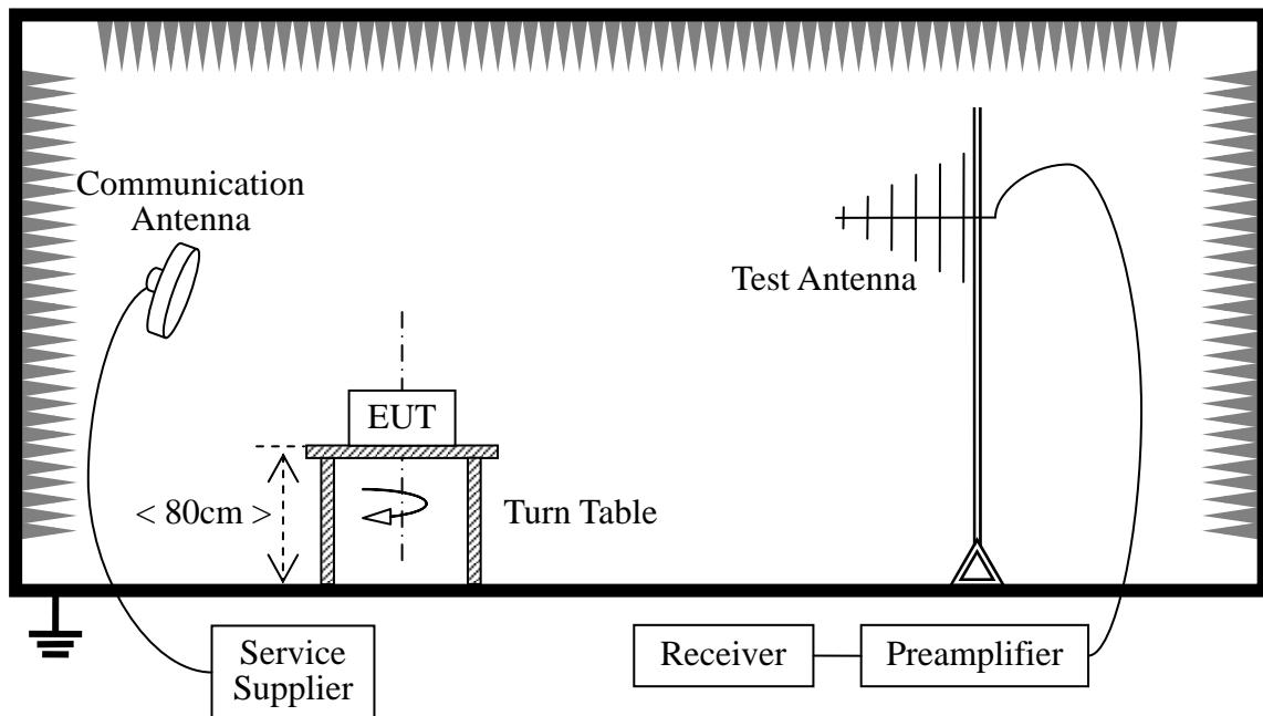
The EUT received AC 120V/60Hz. The Module is located in a 3m Semi-Anechoic Chamber; the antenna factors, cable loss and so on of the site as factors are calculated to correct the reading. During the measurement, the EUT is activated and transmitting with the other WIFI device (Supply by the Applicant) during the test.
