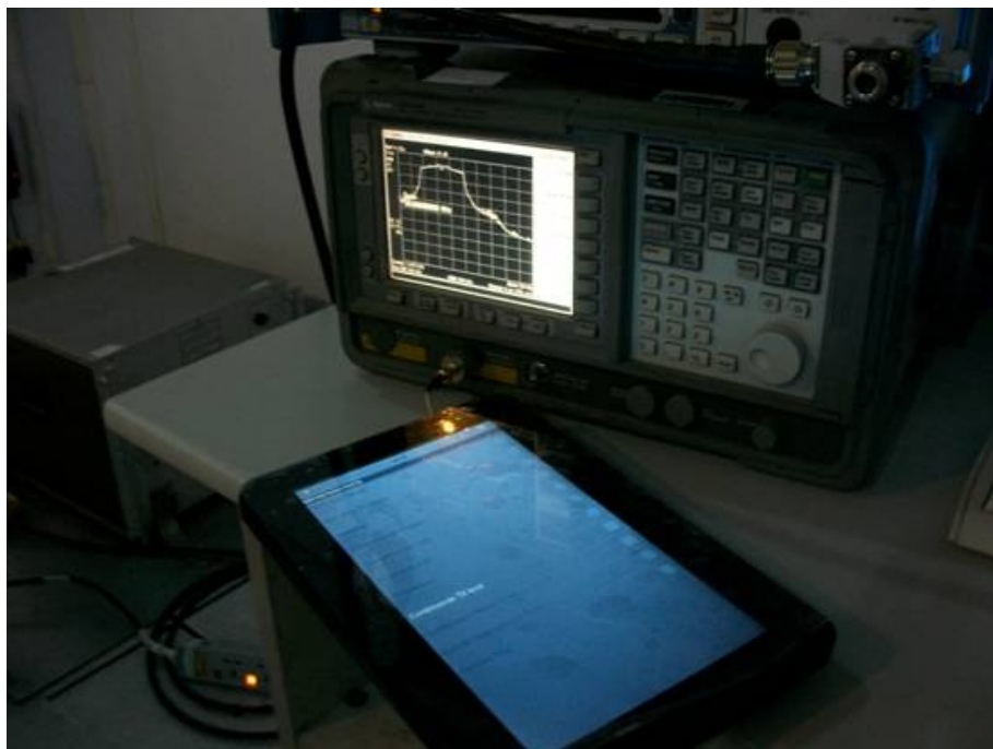
CONDUCTED SPURIOUS EMISSION TEST SETUP
