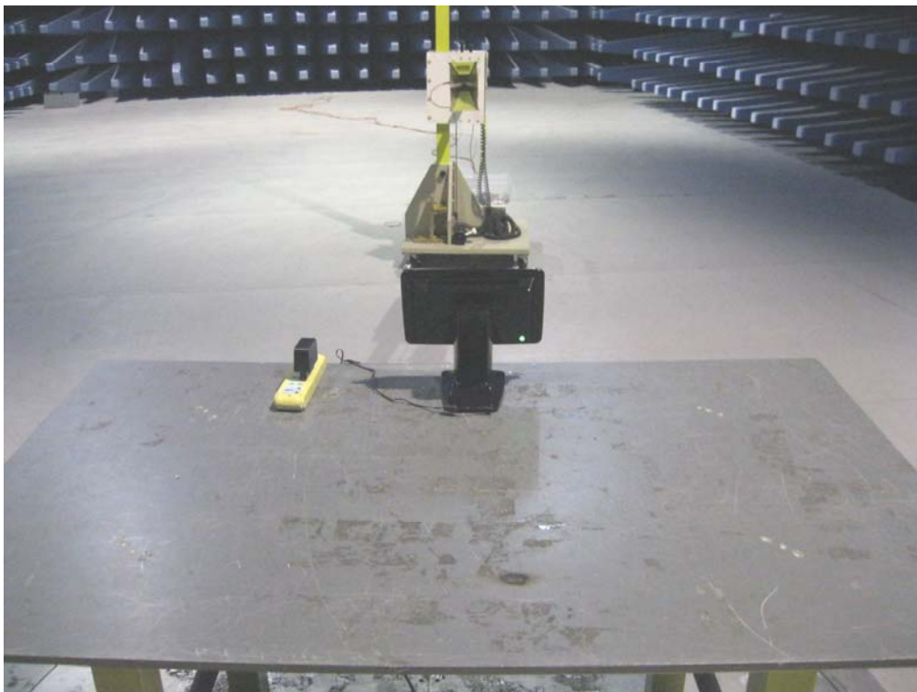
Radiated Spurious Emissions Test Setup (Above 1GHz)
