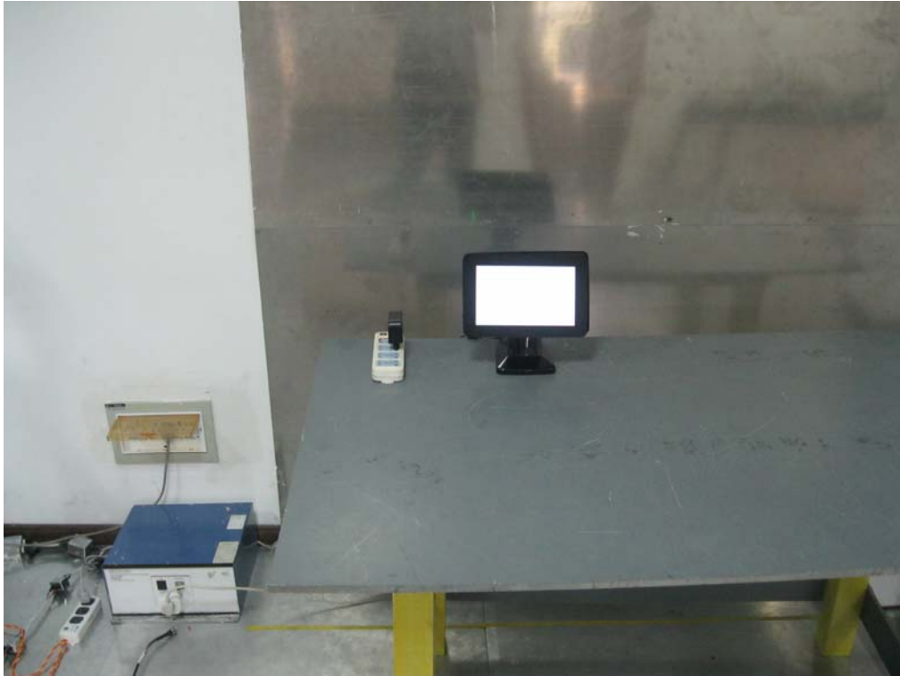
Conducted Emissions Test Setup Front View
