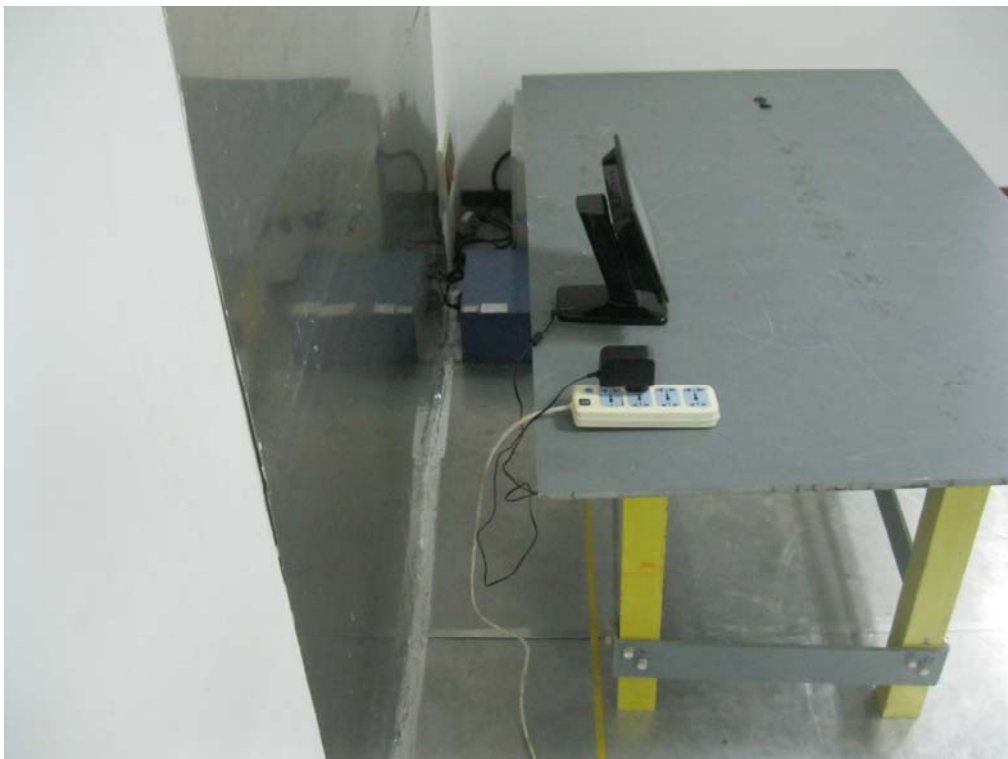
Conducted Emissions Test Setup Side View
