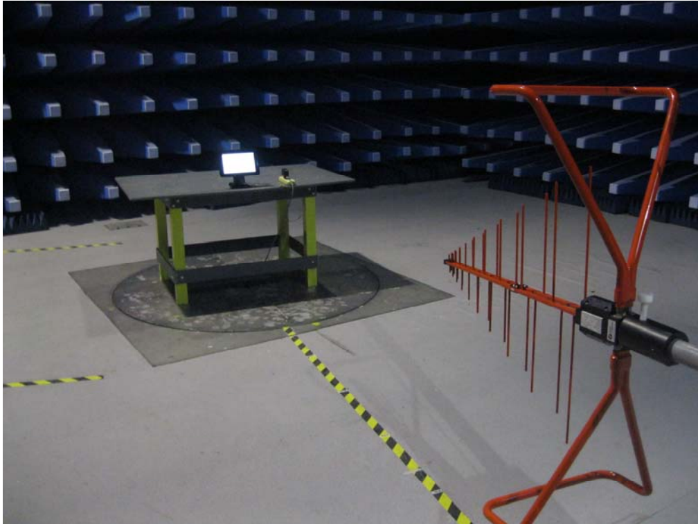
Radiated Spurious Emissions Test Setup (30MHz-1GHz)
