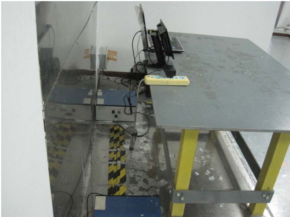
Conducted Emission Test Setup Side View Connected to PC
