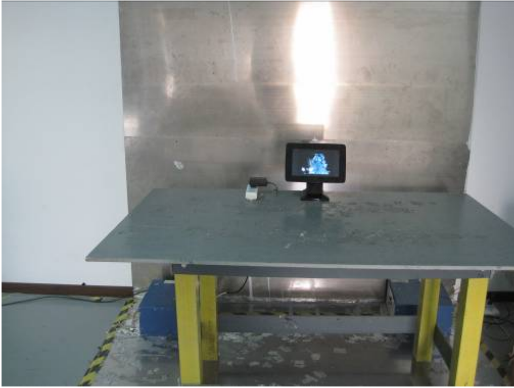
Conducted Emission Test Setup Front View
