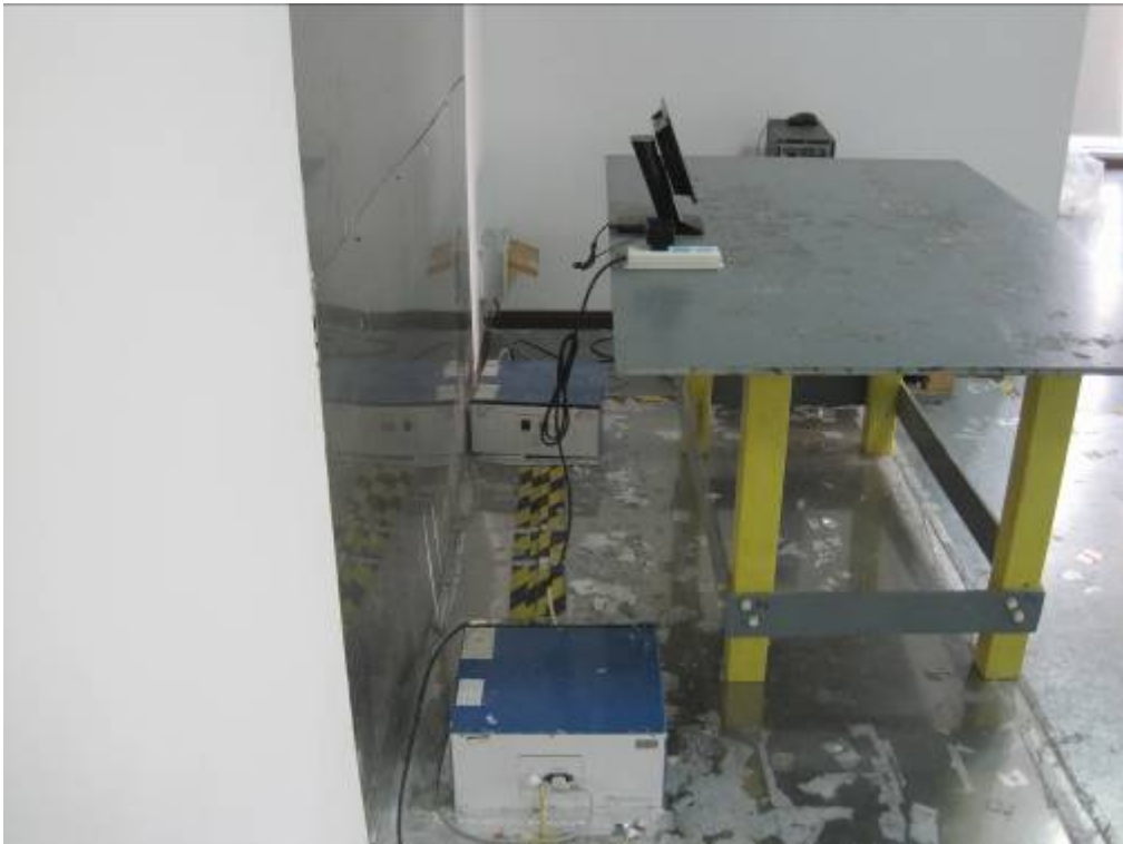
Conducted Emission Test Setup Side View
