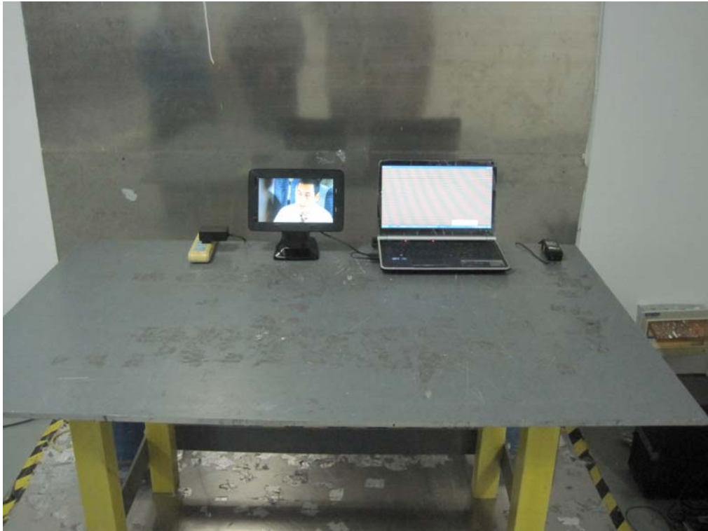
Conducted Emission Test Setup Front View Connected to PC
