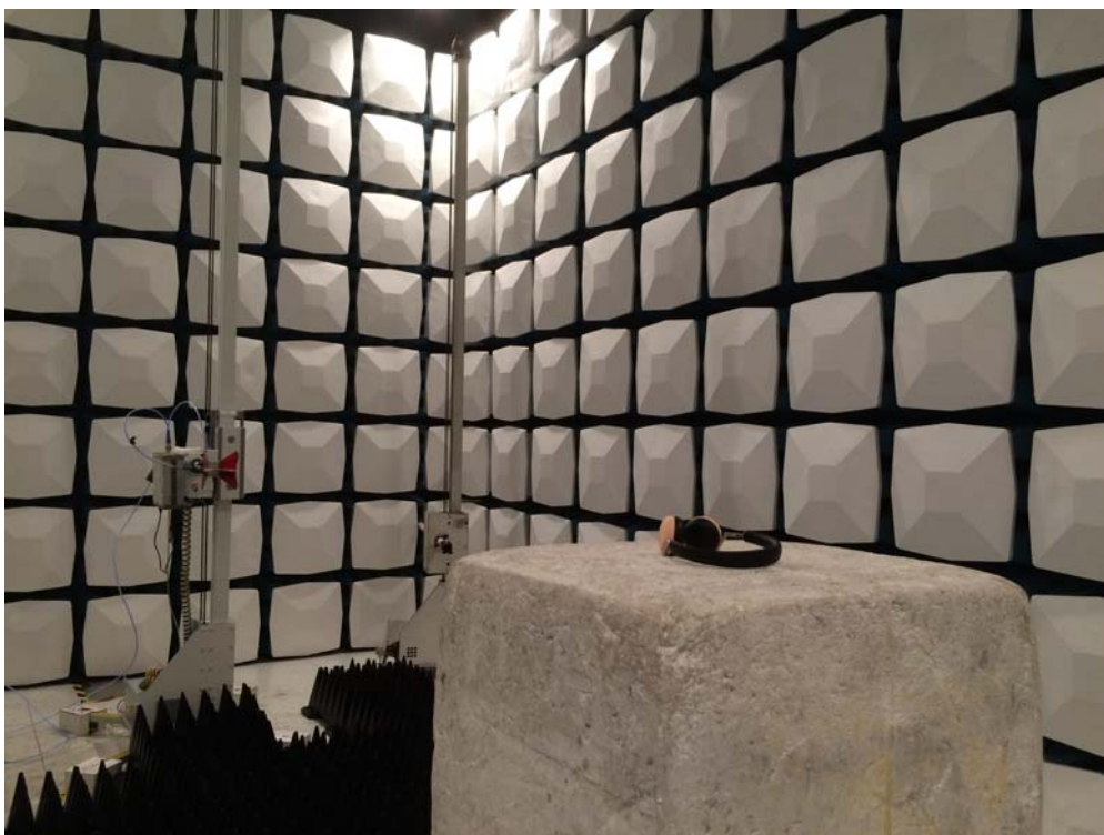
Description: Radiated Emission Test Setup for 1~18GHz
