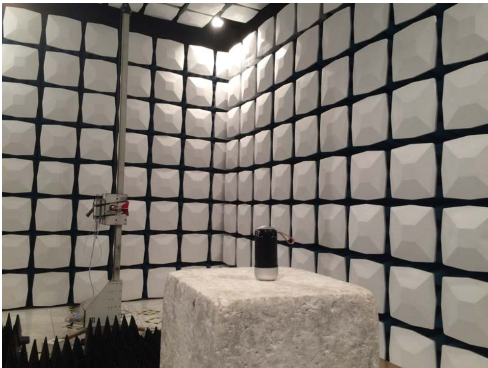
Description: Radiated Emission Test Setup for 1~18GHz
