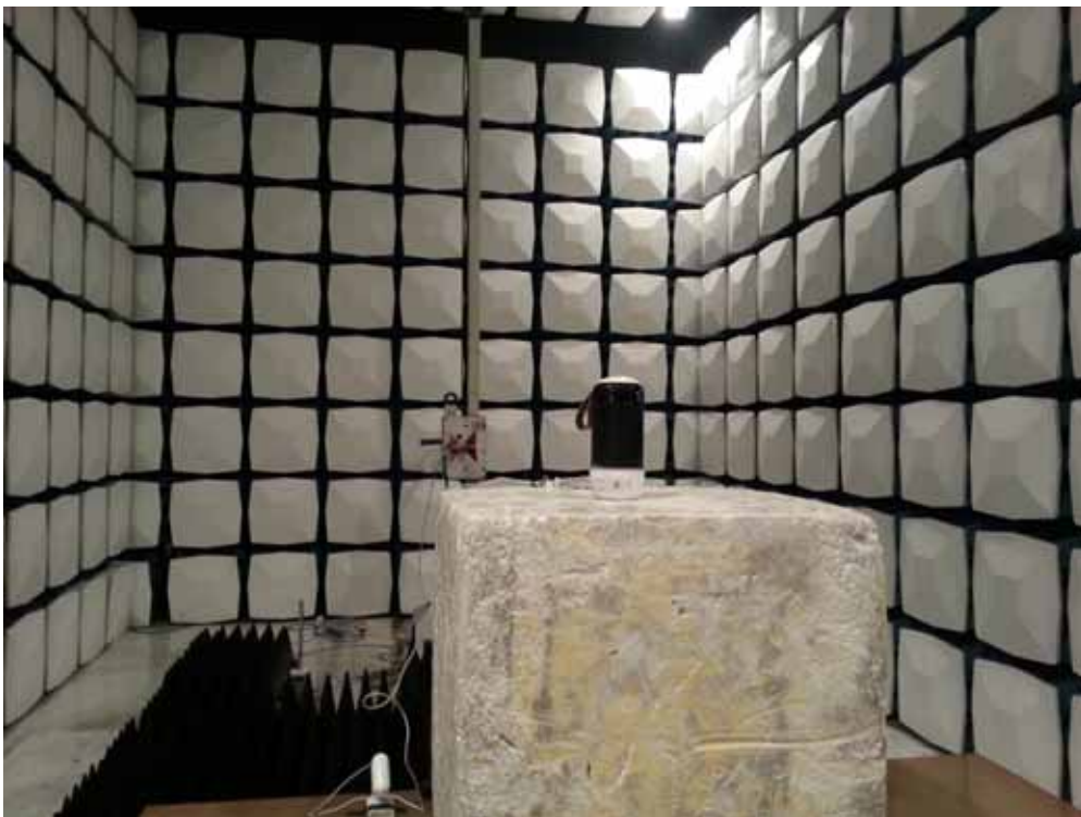
Description: Radiated Emission Test Setup for 1~18GHz
