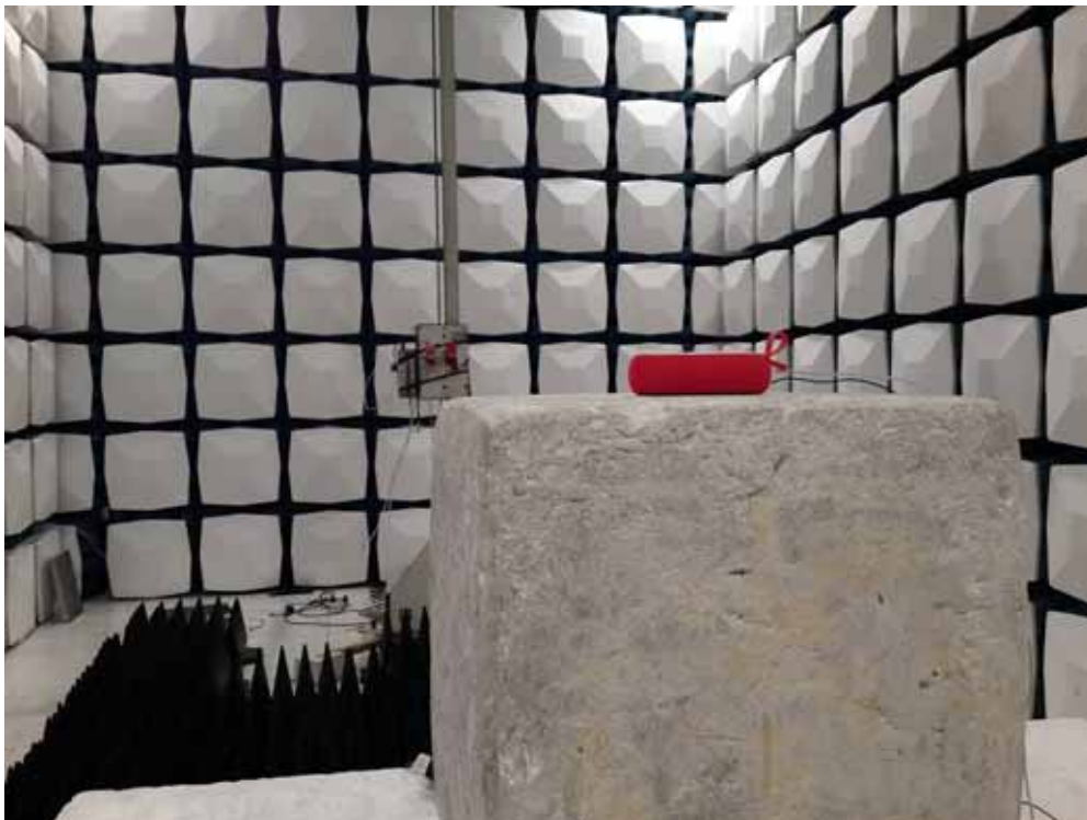
Description: Radiated Emission Test Setup for 1~18GHz
