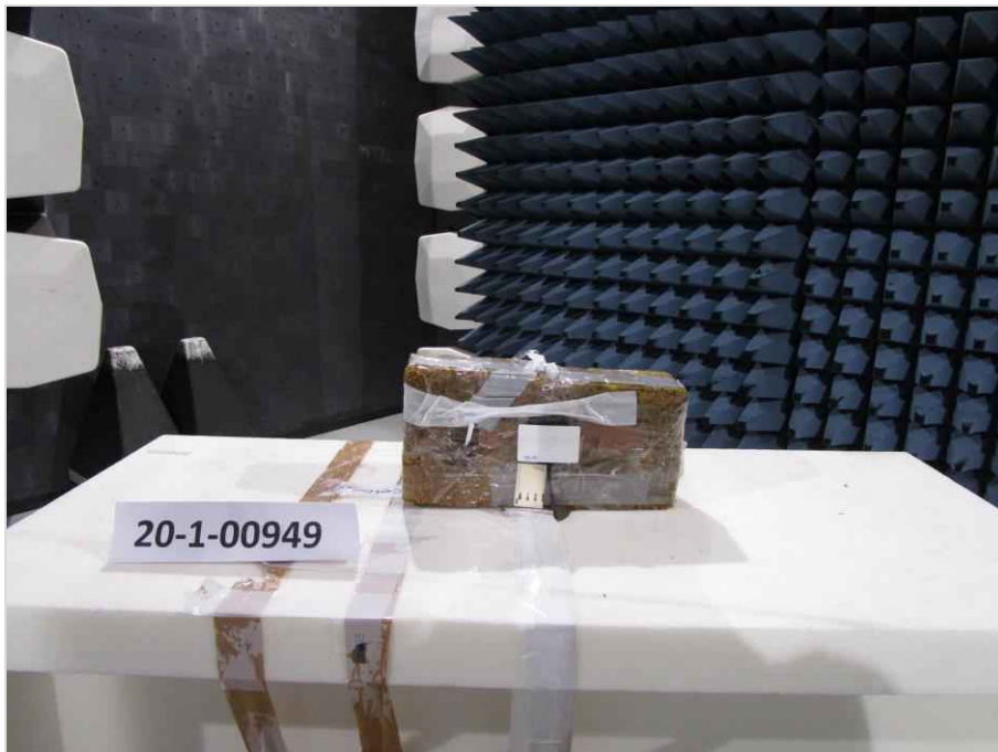
Photograph 7: EUT test setup 2 in the semi anechoic chamber, close up view_EUT elevation 90°
