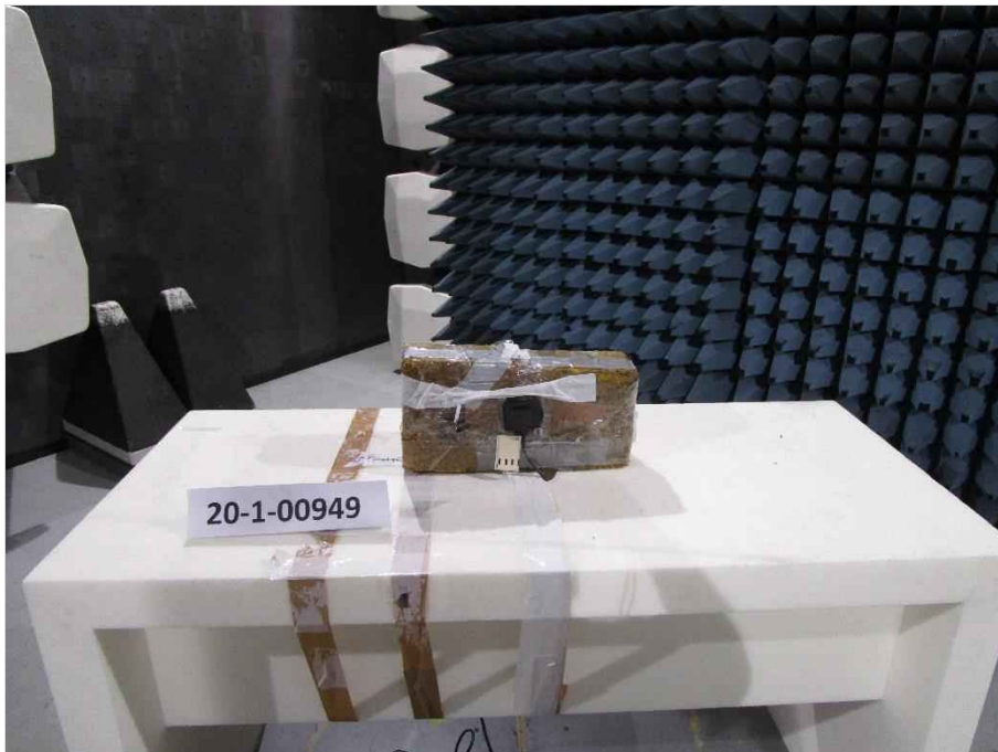
Photograph 3: EUT test setup 1 in the semi anechoic chamber, close up view_EUT elevation 90°
