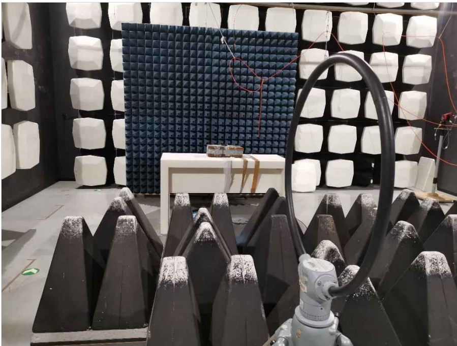
Photograph 10: EUT test setup 1 in the semi anechoic chamber, overview_EUT elevation 0°, EUT in TX mode
