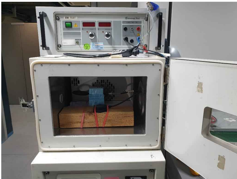
Photograph 14: EUT setup 2 conducted measurement, overview
