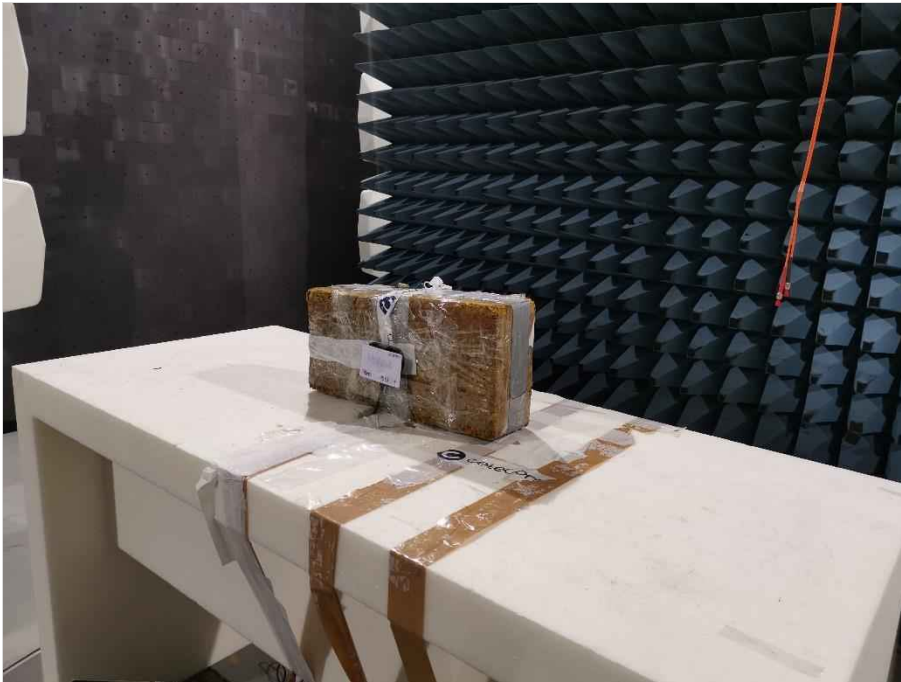
Photograph 11: EUT test setup 2 in the semi anechoic chamber, close up view_EUT elevation 90°, EUT in TXRX mode
