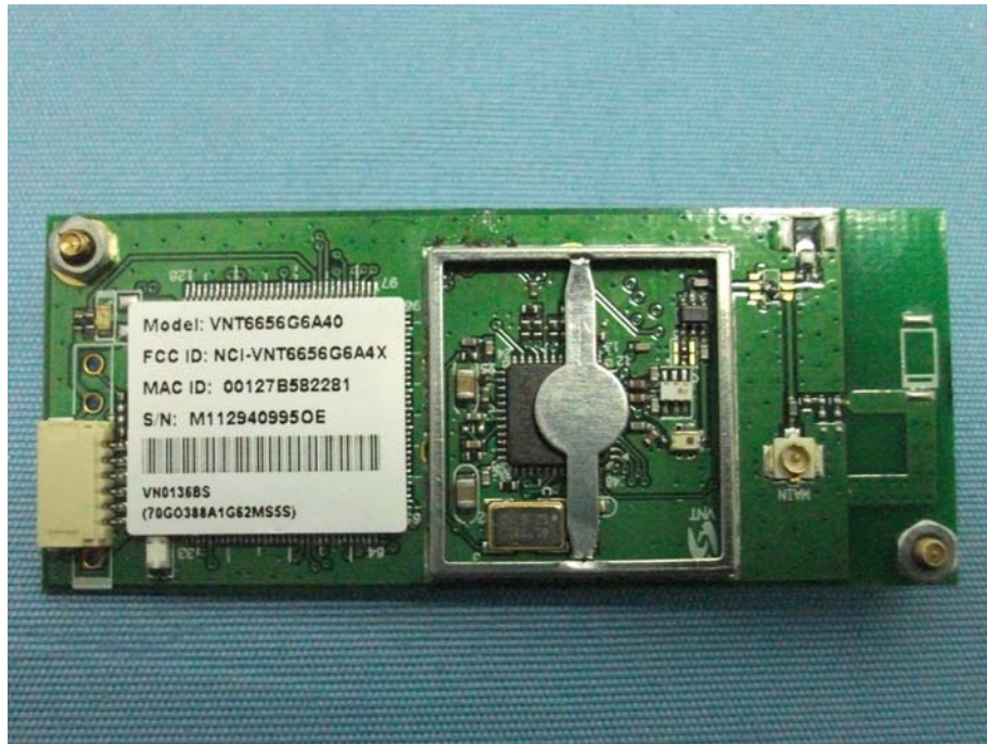
Figure 13 PCB of the EUT-Front View (Un-Shielding)
