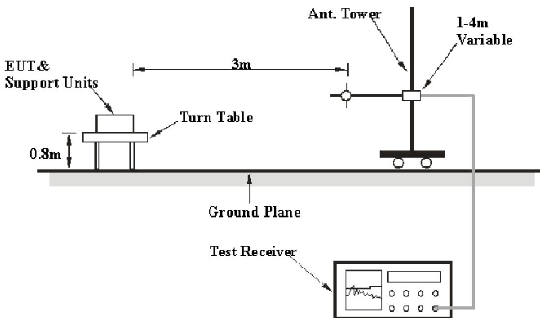
The radiated emission tests were performed in the chamber B test site, using the setup accordance with the ANSI C63.4-2003. The specification used was the FCC Part 15 Subpart C section 15.227 limits.
