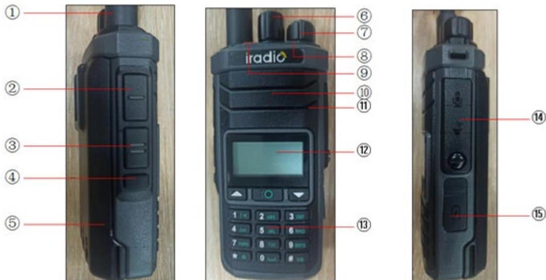
① Antenna ②PTT ③Side-key 1 ④Side-key 2 ⑤Battery ⑥Short/Medium/Long Wave FM Antenna
