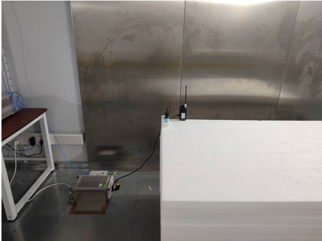
Conducted Emission_Side View(Mode 1)
