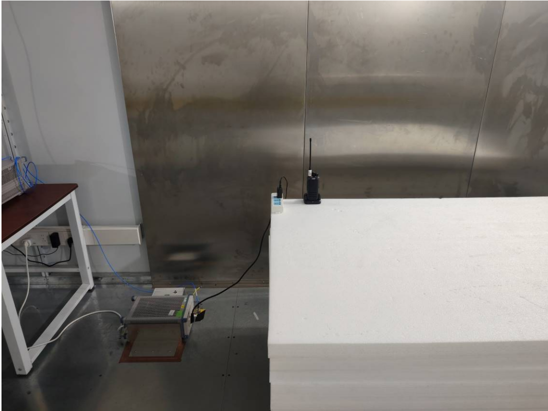
Conducted Emission_Side View(Mode 3)
