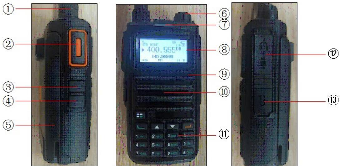
①Antenna ②PTT ③Side-key1 ④Side-key 2 ⑤Battery ⑥ON/OFF/Volume Knob ⑦Indicator ⑧ Display ⑨MIC
