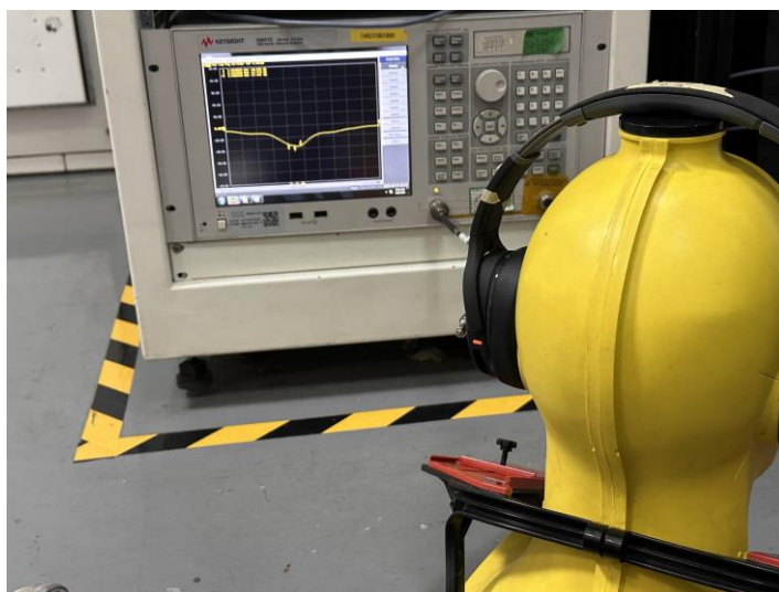
Free Space Impedance Setup
