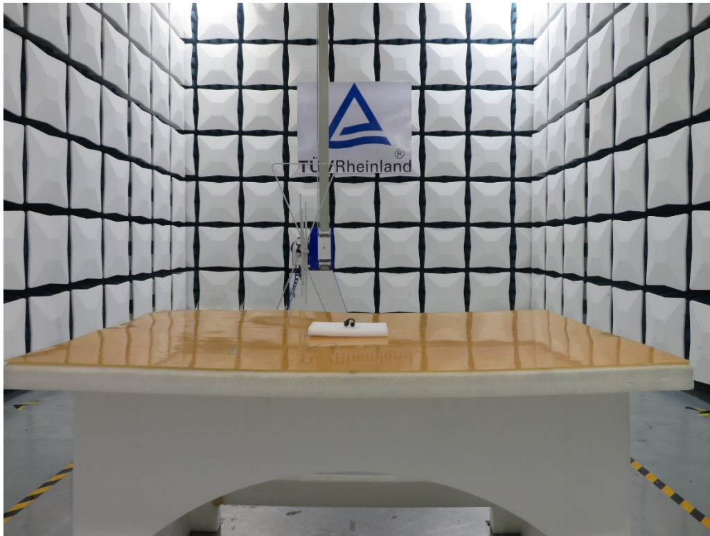
Photograph 1: Set-up for Radiated Spurious Emission, Below 1GHz
