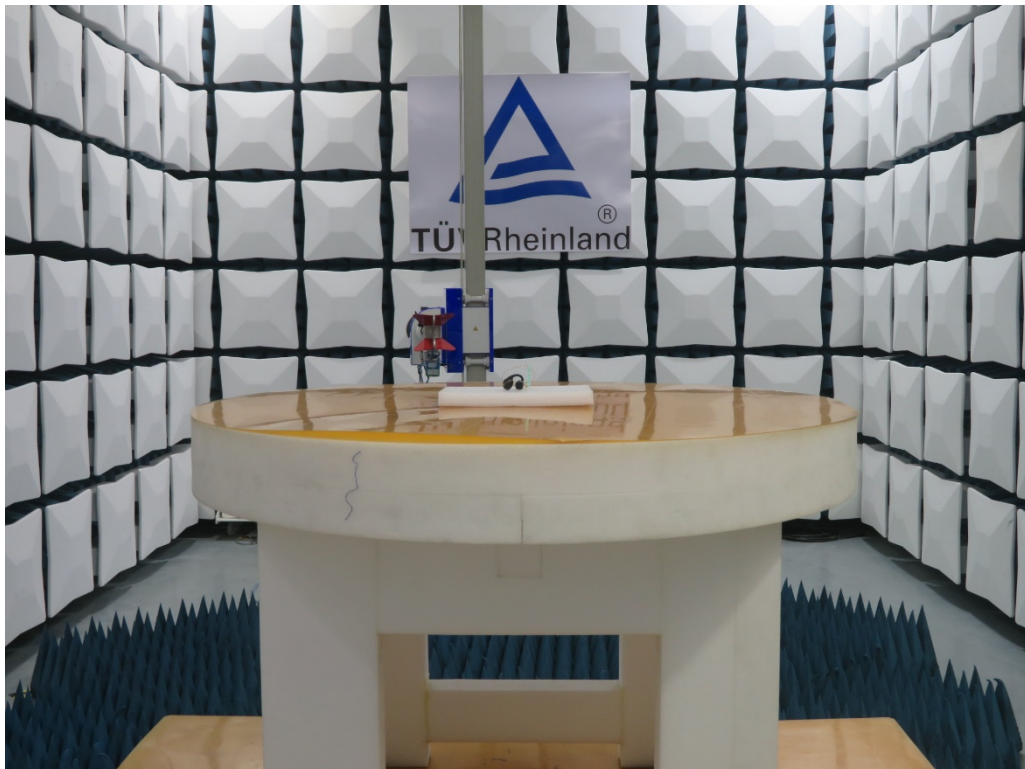
Photograph 2: Set-up for Radiated Spurious Emission, Above 1GHz
