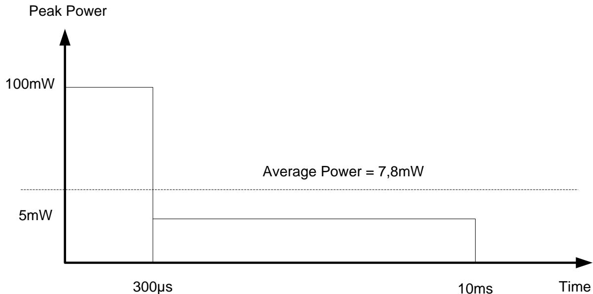
The diagram shows one cycle of the worst case power profile running the OMR-WAVE-UNIT with the user application. The profile can be repeated several times, but this does not affect the average value. It shows that the transmitted peak power is 100mW for maximum 300µs. The rest of the time the unit transmits not more than 5mW. The average power for the whole transmission is less than 7,8mW.
