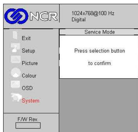
After picture adjustments have been optimized, the settings are memorised automatically. The OSD menu will disappear after 10 seconds of inactivity (timeout adjustable through the OSD menu) or the OSD can be exited by selecting EXIT.
