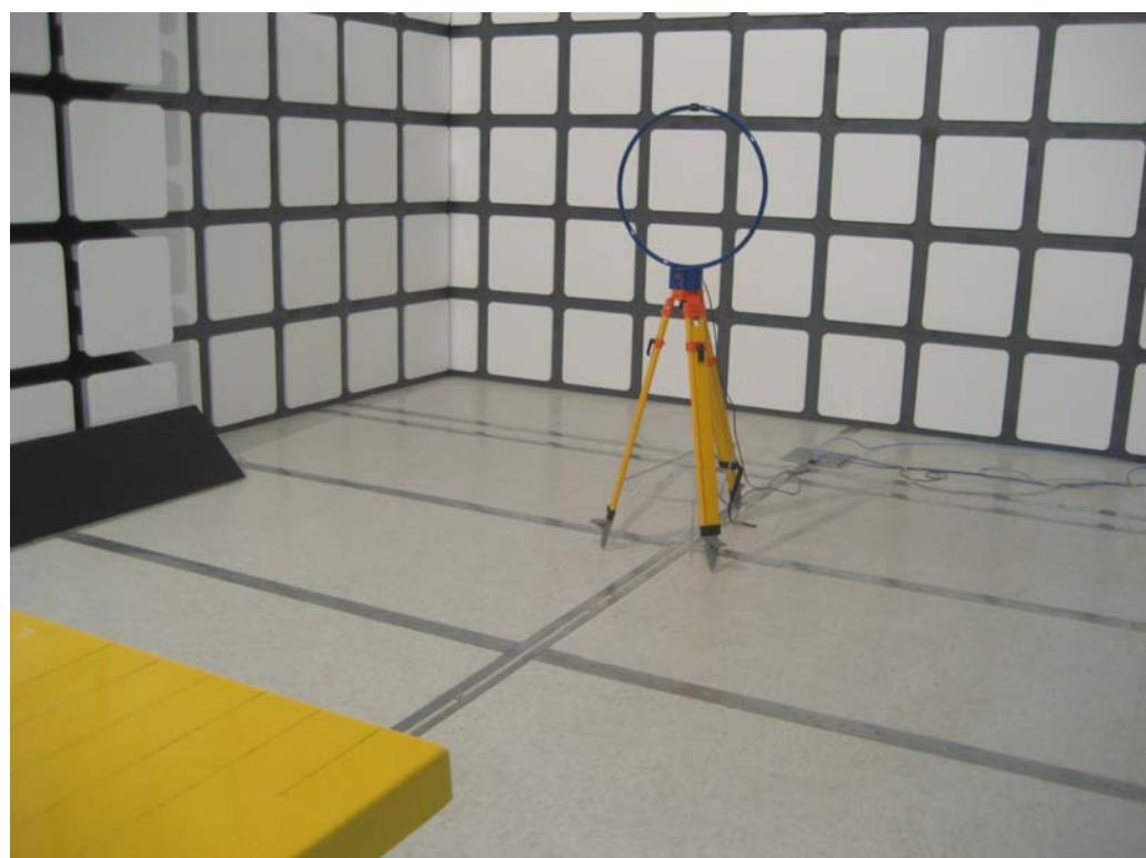
**Test Configuration: 30MHz~1GHz**
