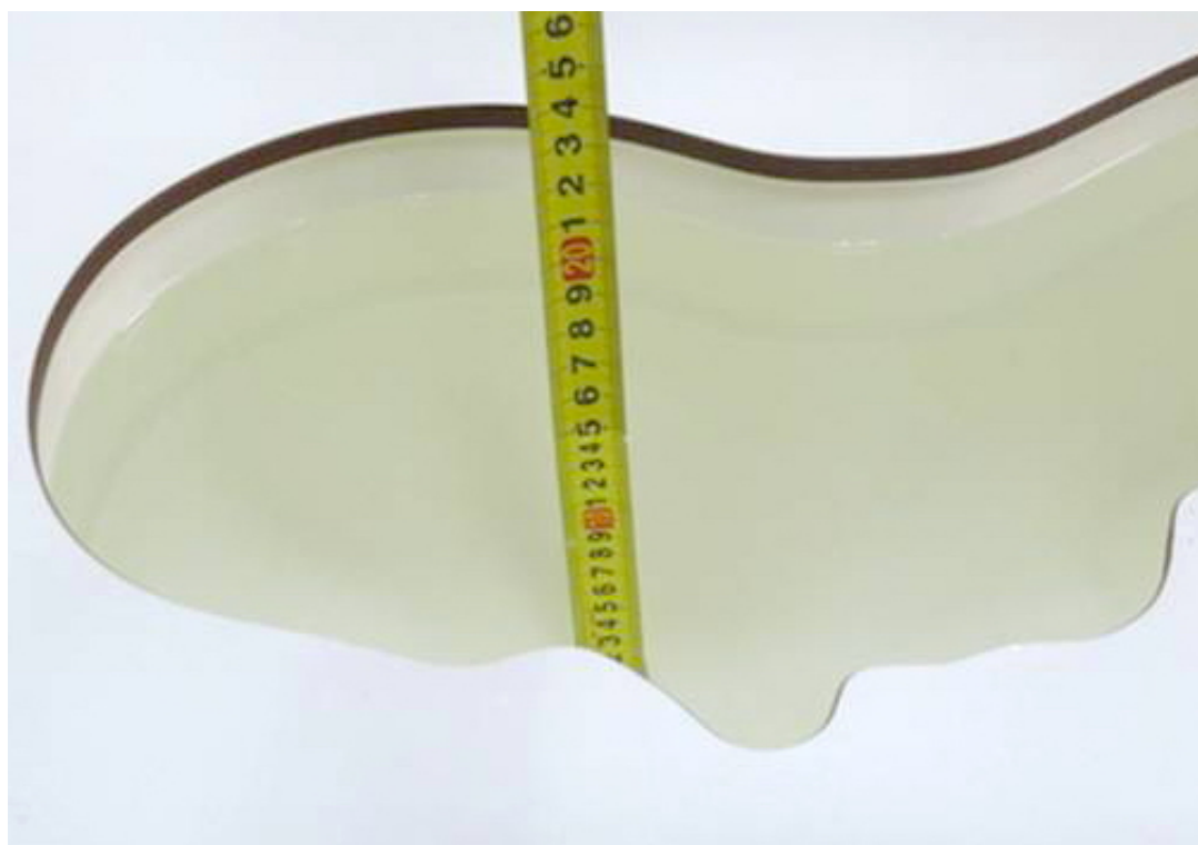
Picture 4: liquid depth in the head Phantom (1800 MHz)
