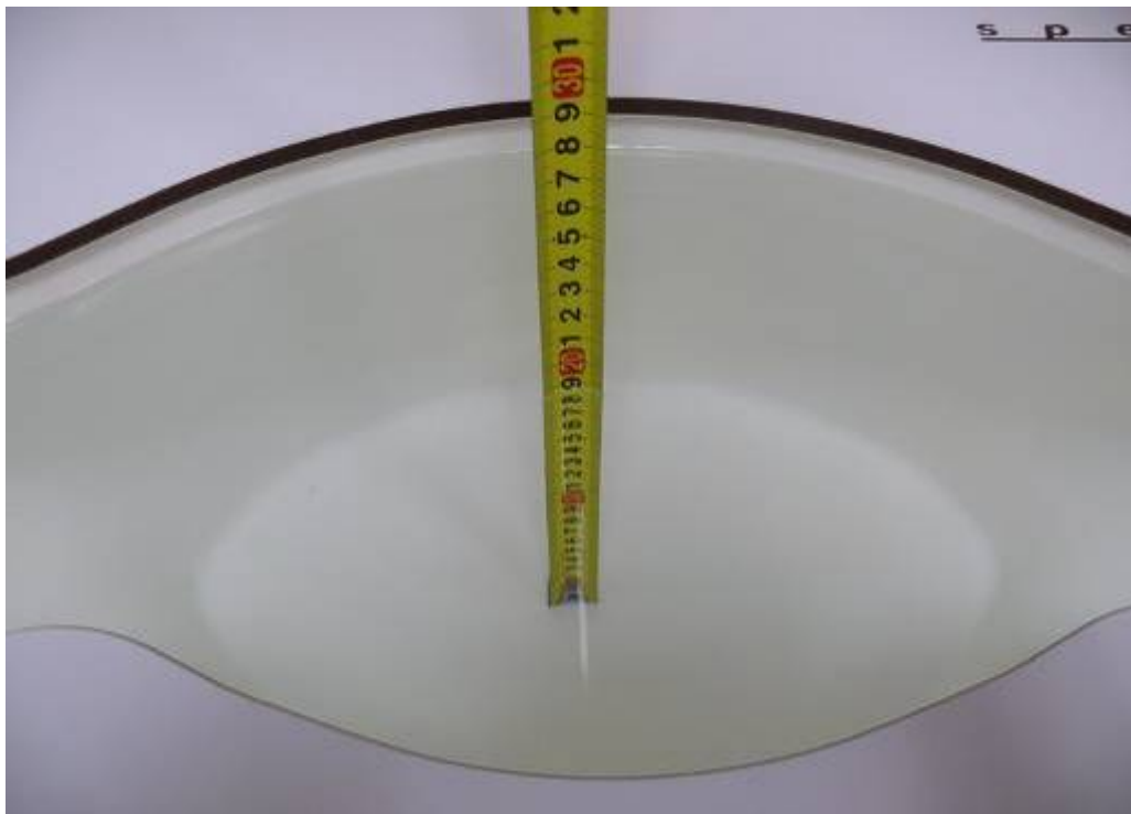
Picture 5: Liquid depth in the Flat Phantom (1800 MHz)
