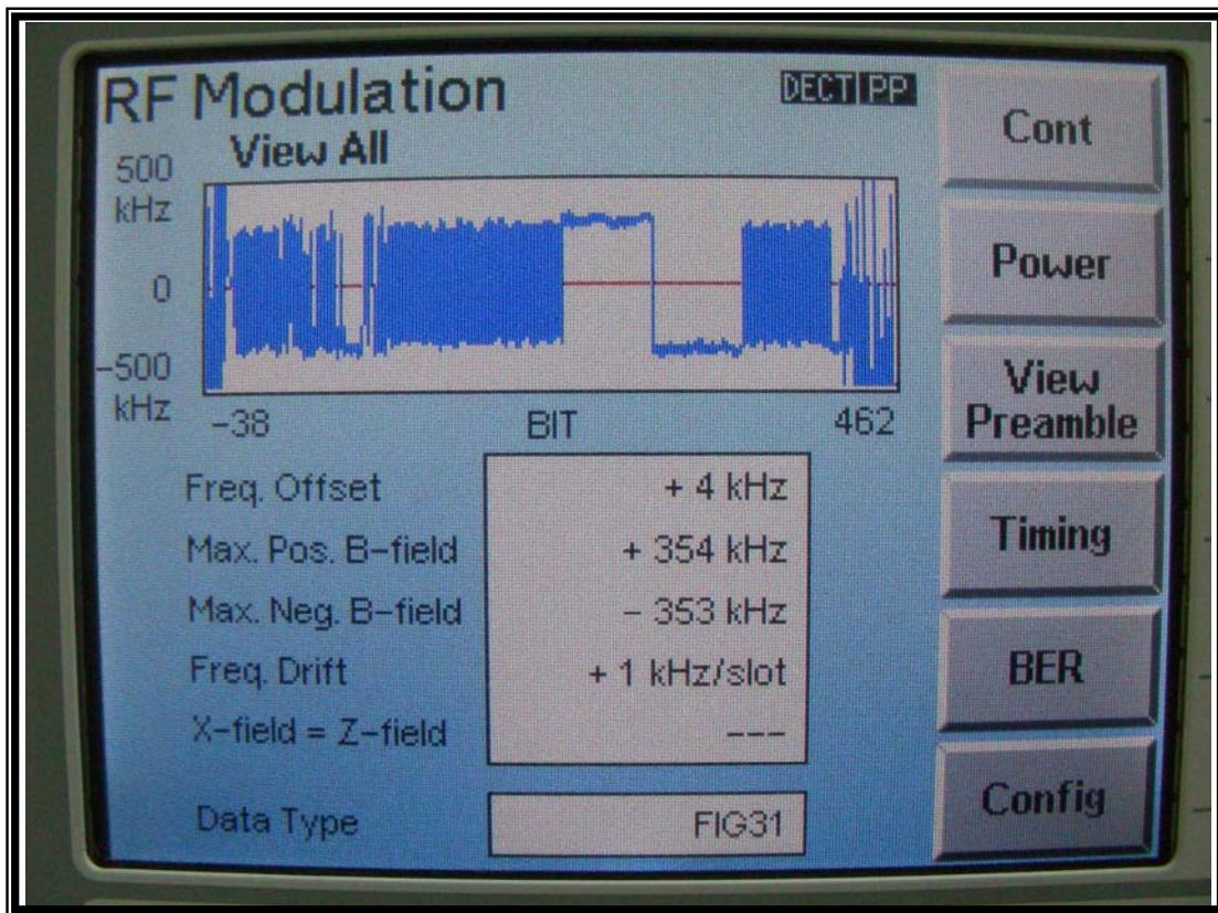
b) Carrier Frequency Stability over temperature
