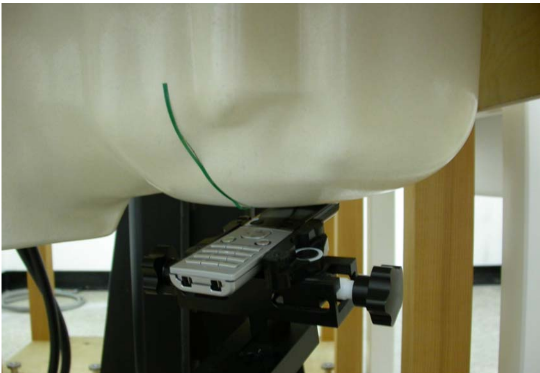
Measurement Position of Left-Tilt (LT) with Handset
