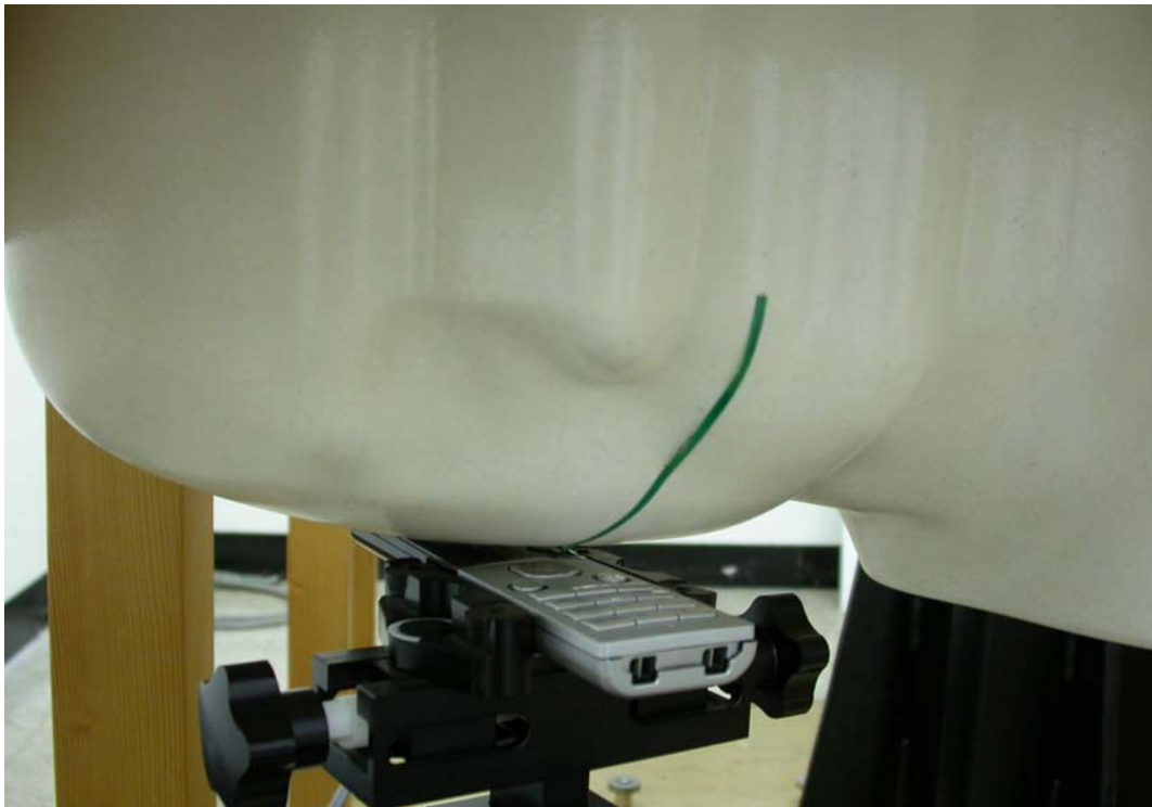
Measurement Position of Right-Cheek (RC) with Handset
