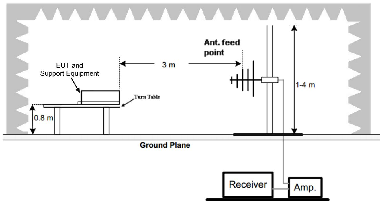
**(B) Radiated Emission Test Set-UP Frequency above 1GHz**
