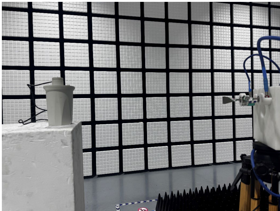
Description: Radiated Emission Test Setup (Above 18GHz)
