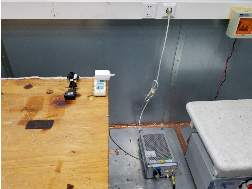
Picture 2: Conducted Emissions Test Setup
