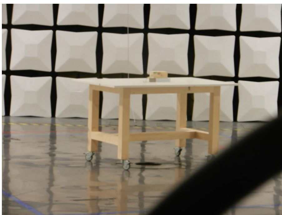
Figure 75 – Test Setup for frequencies 9 kHz – 30 MHz
