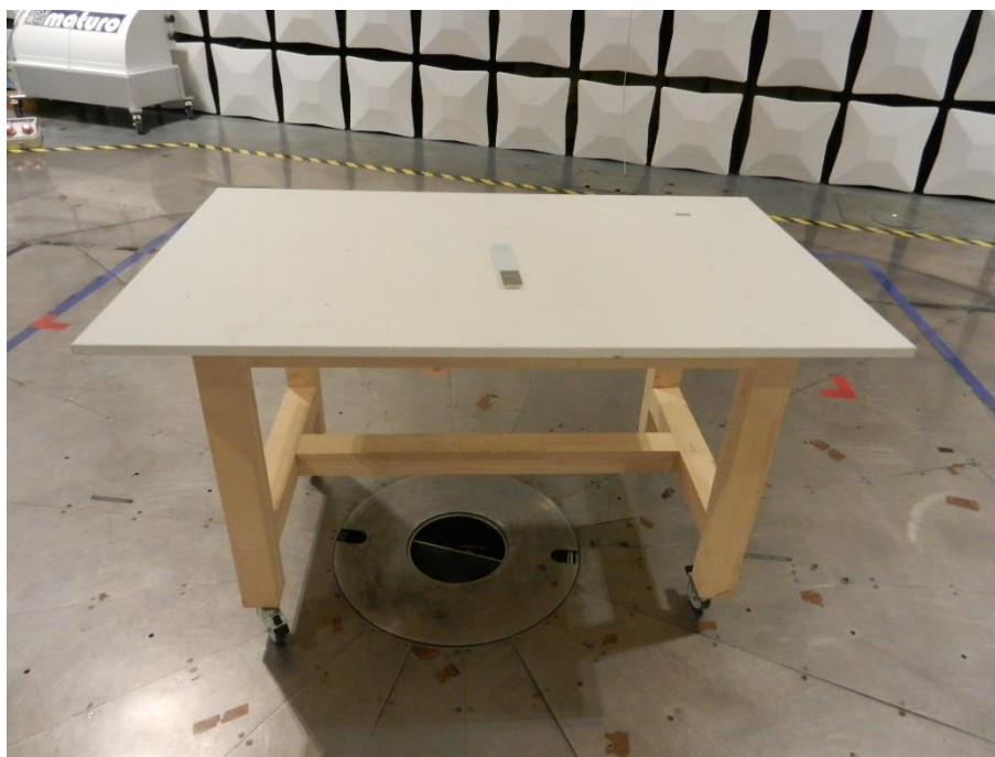
Figure 72 – Test Setup for frequencies 9 kHz – 30 MHz
