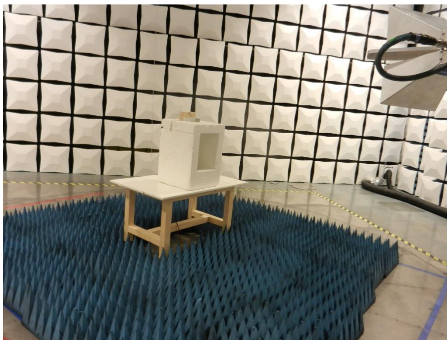
Figure 82 – Test Setup for frequencies >1 GHz
