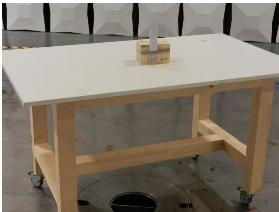
Figure 76 – Test Setup for frequencies 9 kHz – 30 MHz
