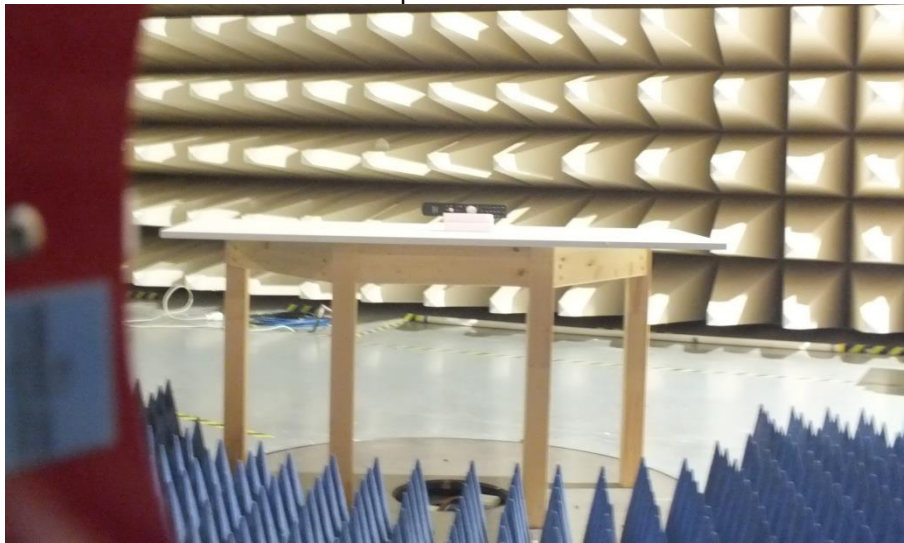
Test setup 1 GHz – 18 GHz:
