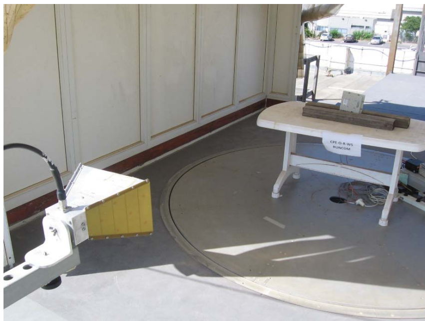
Figure 6. Spurious Radiated Emission Test – 1-7GHz
