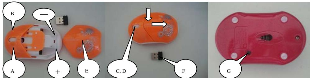
A; left button   B; right button   C.D; scroll wheel   E; battery shell   F; nano receiver   G; ID switch
