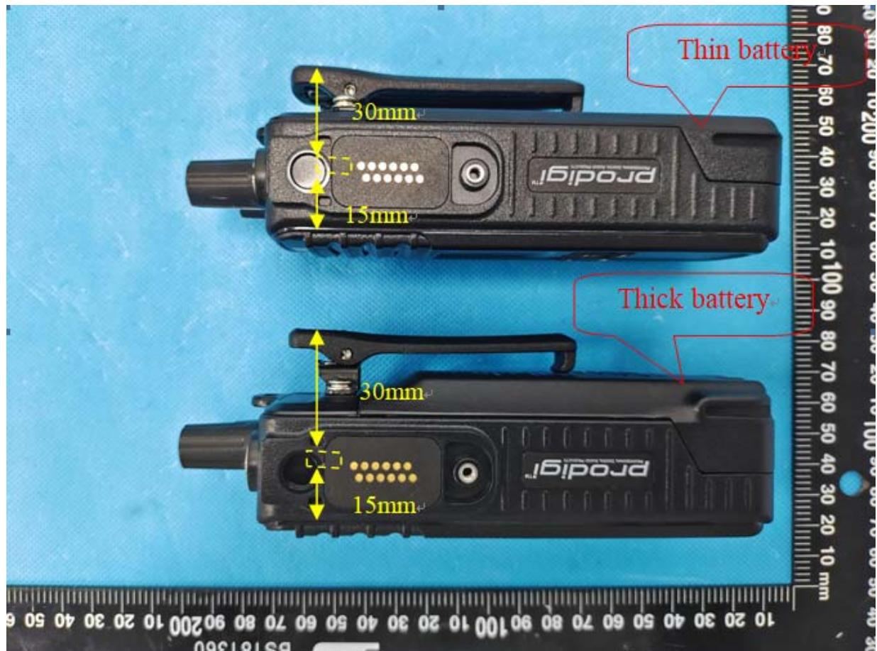
Note: the distance for Body Back(30 mm), for Face Up(15mm+25mm=40 mm)
