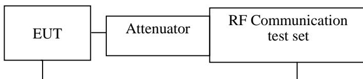
Path loss: 30dB attenuator +1dB lable loss, that total 31dB added into offset.
