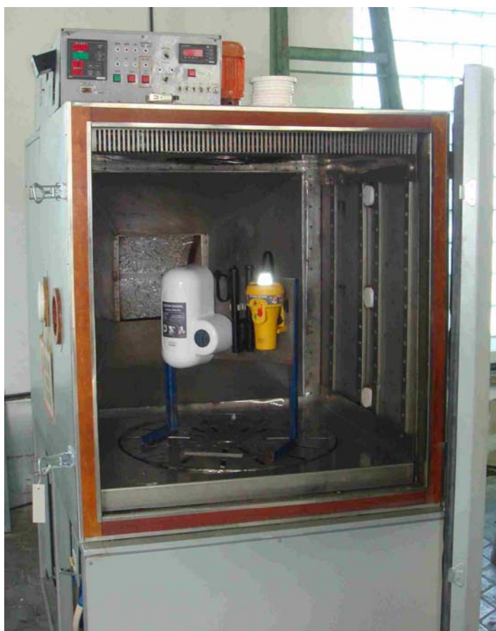
Photo 2 – ARH100 and EPIRB in solar chamber
