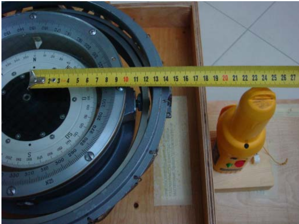
Photo 32. Defining a safe distance from the SART to the main ship's magnetic compass. SART in stand-by mode.
