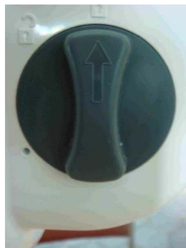
Photo 5 – ARH100 manual release switch after test
