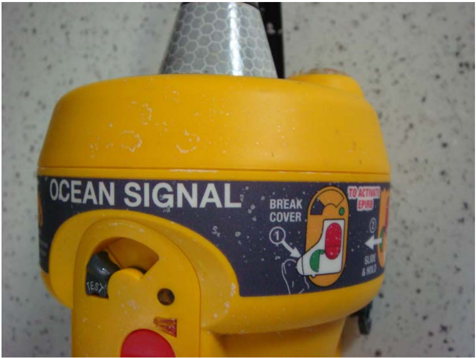
Photo 3 – EPIRB E100G class 2 Category 2 label after test
