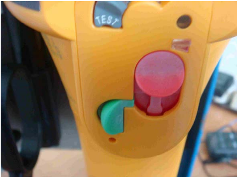
Photo 8 – EPIRB control switches after test
