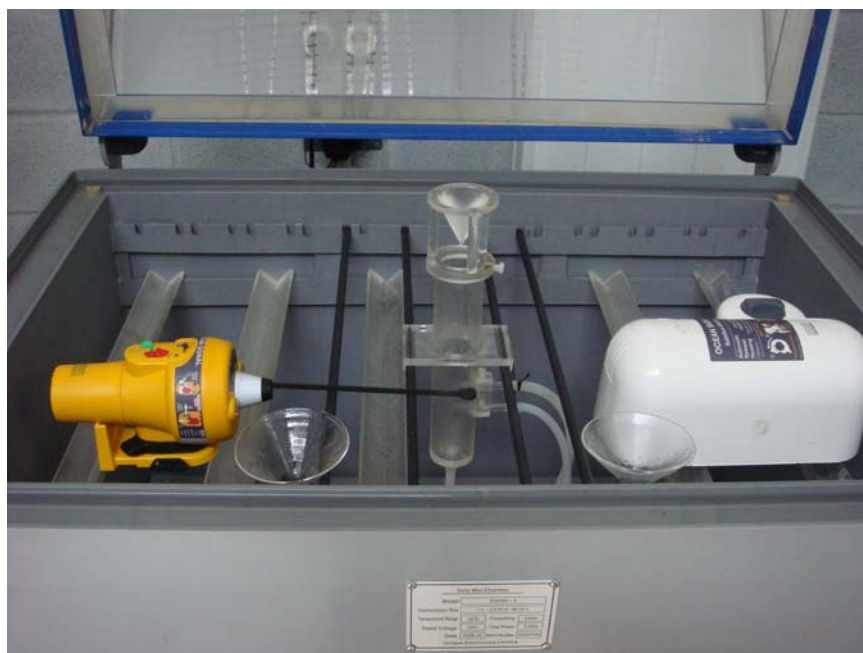
Photo 1 – EPIRB E100G class 1 Category 1 and EPIRB E100G class 2 Category 2 in salt fog chamber
