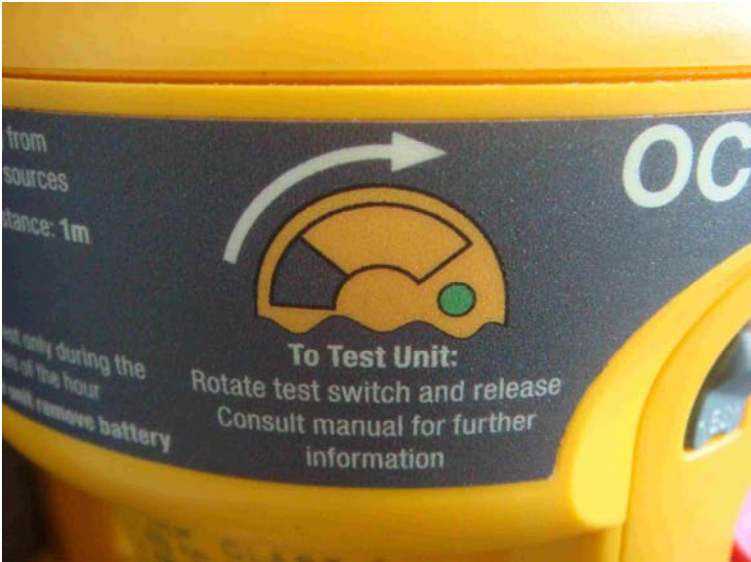
Photo 7 – EPIRB label for selftest after test
