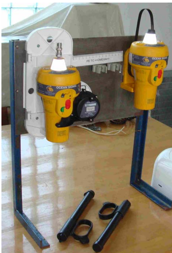
Photo 1 – Prepare ARH100 with EPIRB to test
