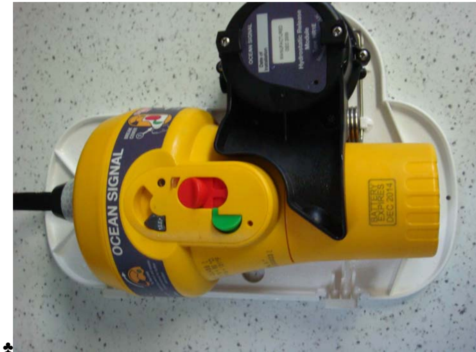
Photo 5 – EPIRB E100G class 1 Category 1 without cover after test
