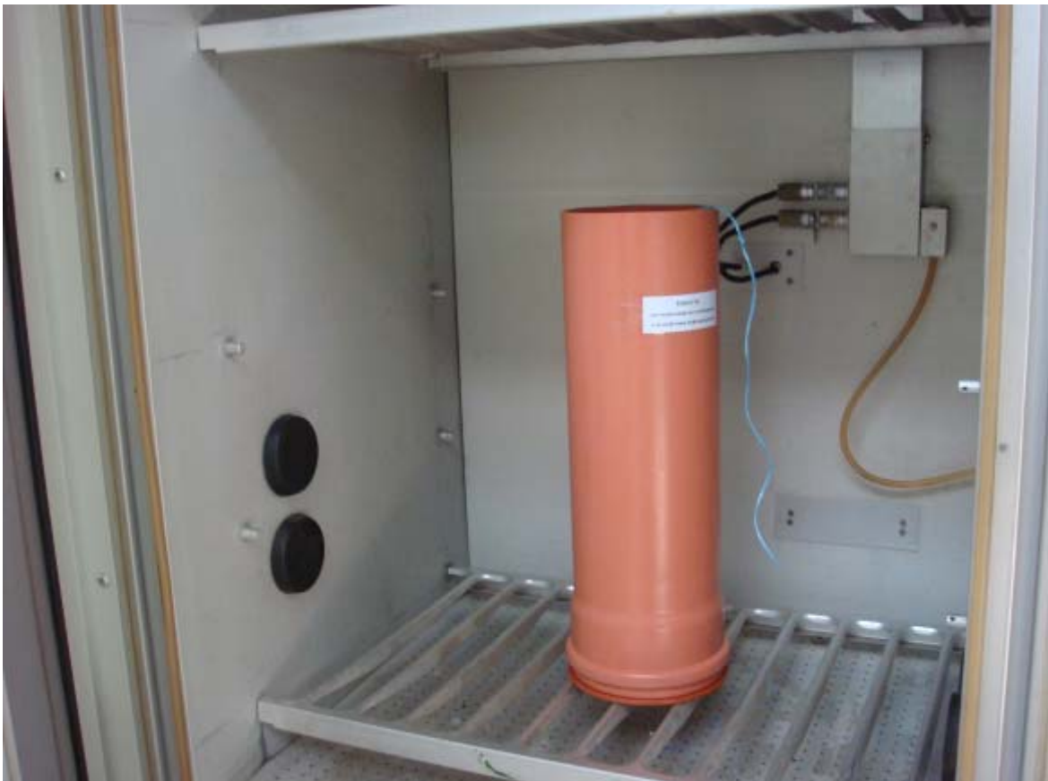
Photo 35 — Tank with oil in temperature chamber
