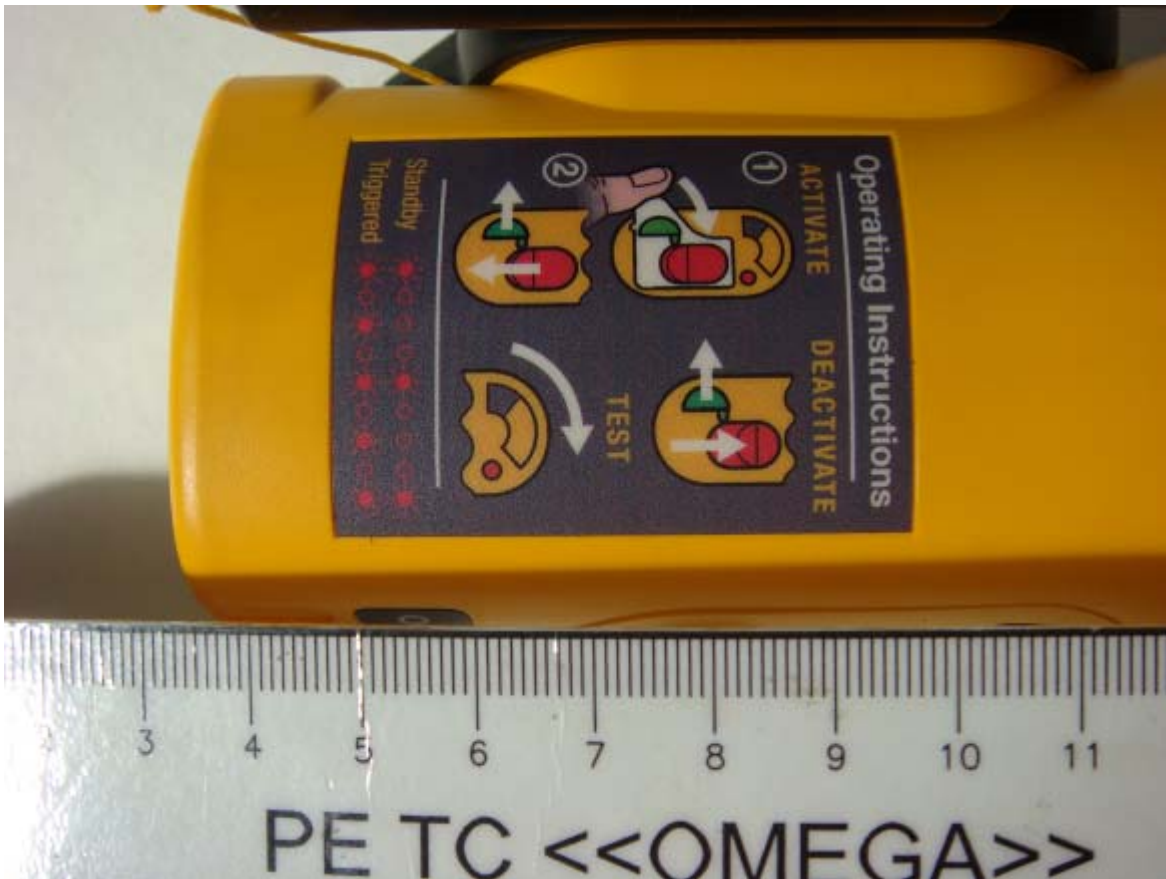
Photo 37— Labeling of SART after oil resistance test.
