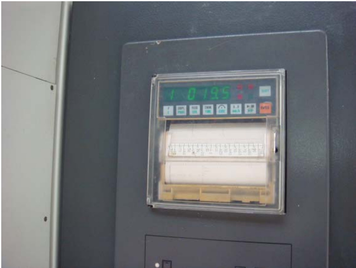
Photo 36— SART in temperature chamber. Temperature +19.5 °C
