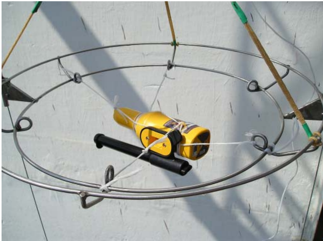
Photo 25 – Dropping of the sample. The antenna position to the side.
