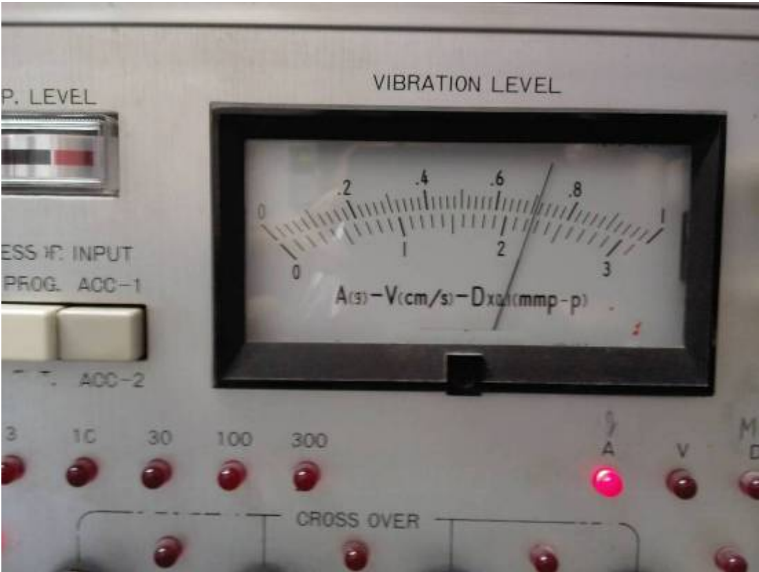
Photo 18 – Indications on the display of a given acceleration. 0,7g
