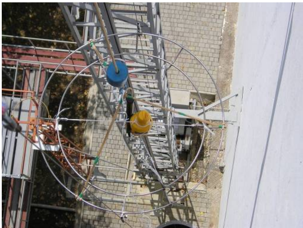
Photo 21– Point for drop test into the water from a height of 20.1 m. Pole is attached.
