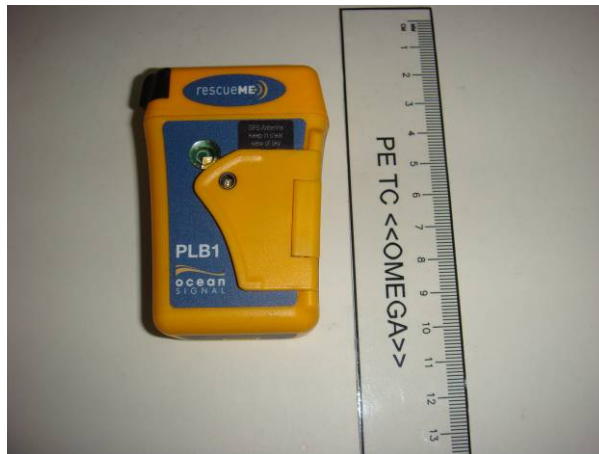
Figure 8.2 – View of the EUT upon completion of the Thermal shock test.
