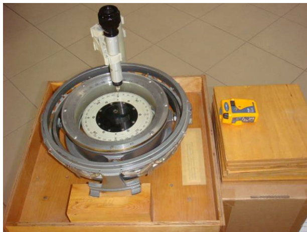
Figure 18.2 - The safety distance from EUT in stand-by mode to standard compass is 0,21 m.
