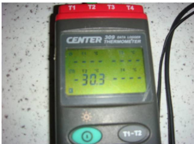
Figure 7.1 - Detailed measurement of the EUT temperature before the drop test
