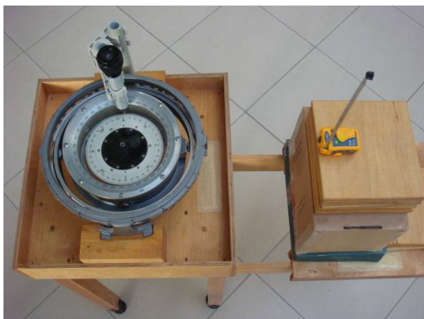
Figure 18.5 - The safety distance from EUT in operation mode to standard compass is 0,32 m.
