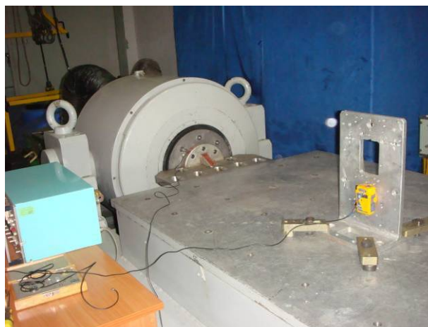
Figure 5.5 - General view of the horizontal Y vibration test
