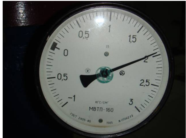
Figure 9.2 –Manometer of immersion test site shows 1,95 bar.
