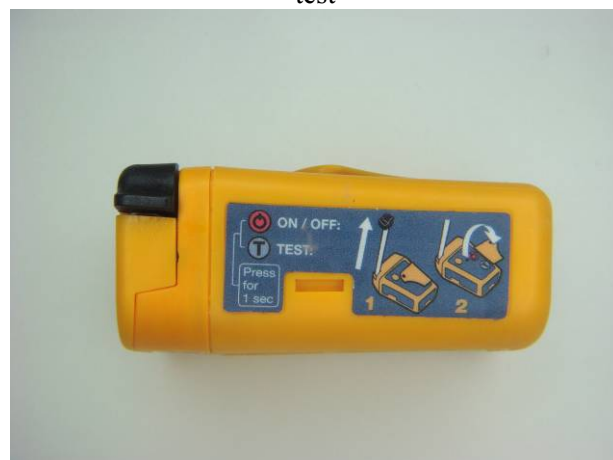
Figure 7.8 - View EUT upon completion of the drop test
