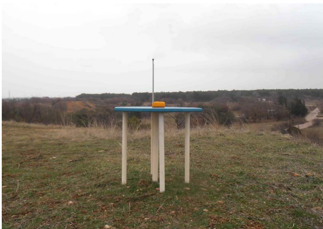
Fig. 11.12 — Satellite qualitative test (Configuration 8 - Beacon above ground plane).
