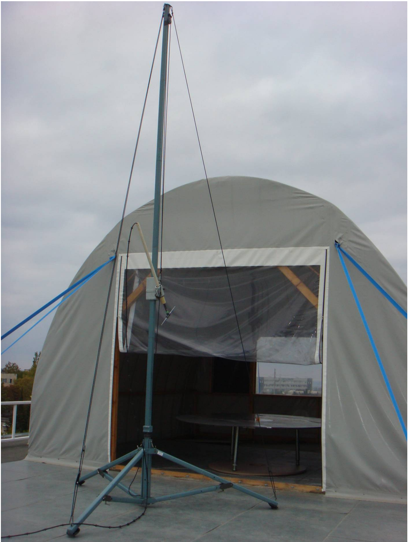
Fig. 11.9 — General view of antenna test place at configuration 3 (section 4.5 standard T.007).i.e. beacon sitting on ground plane.
