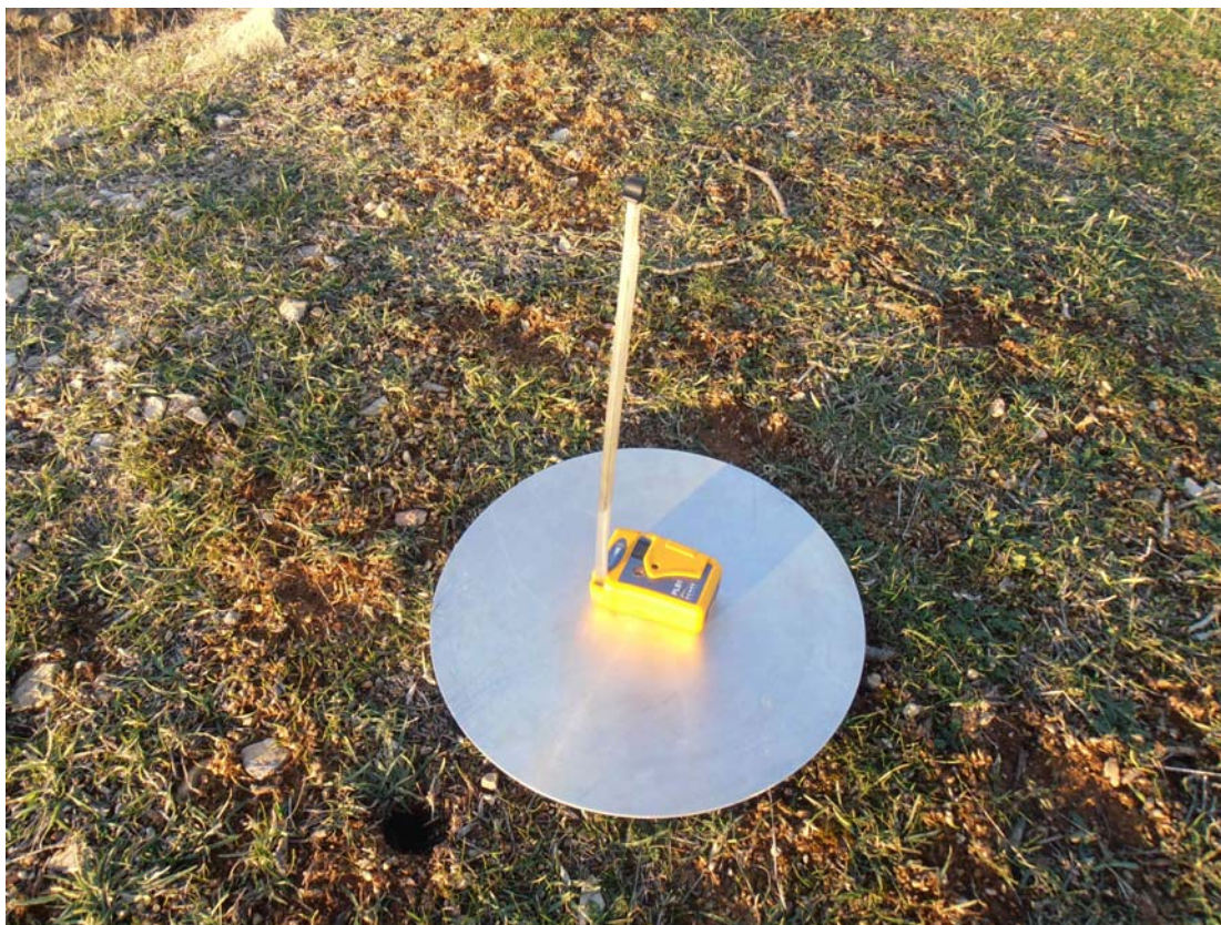
Fig. 11.11 — Satellite qualitative test (Configuration 7 – Beacon on ground plan).
