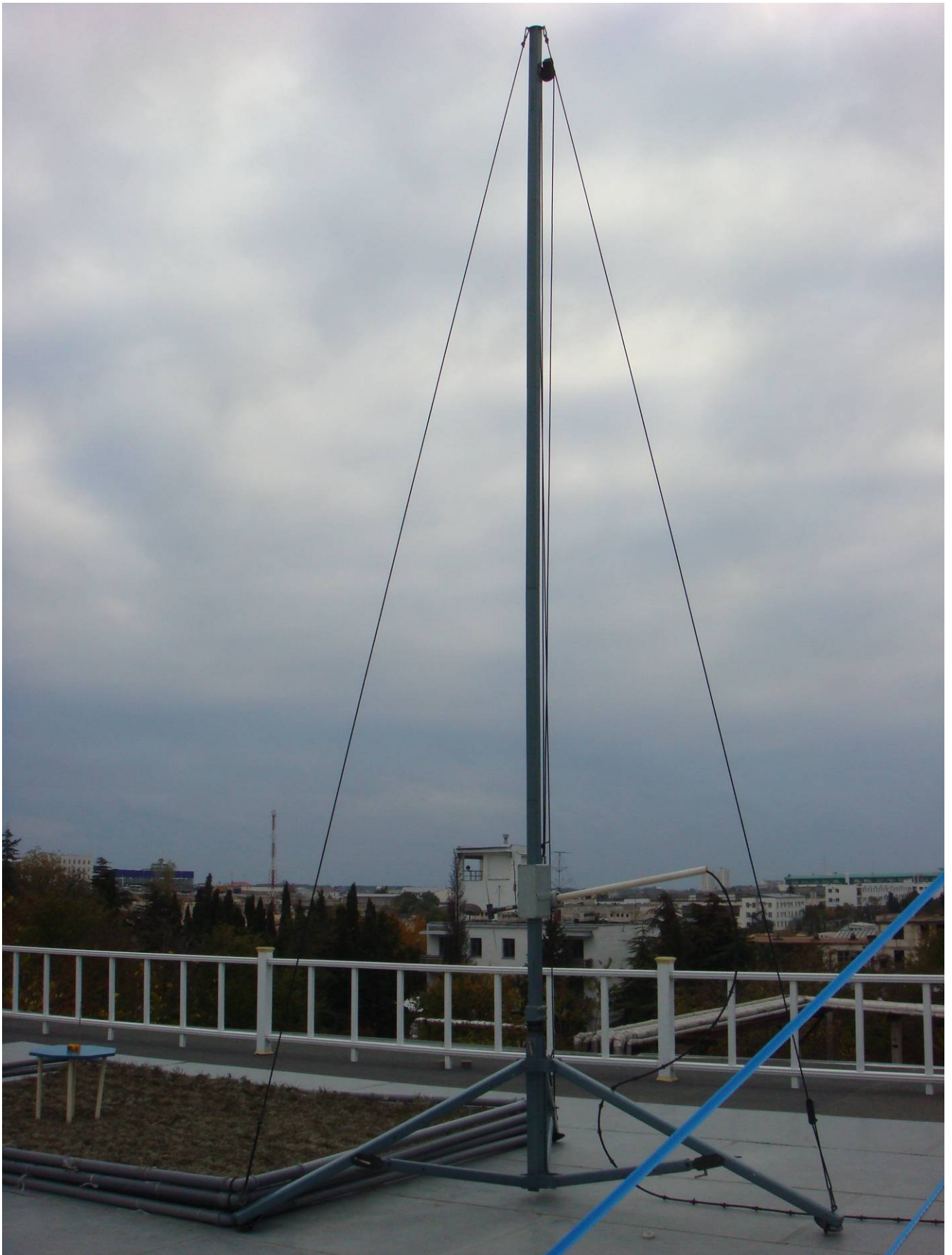
Fig. 11.10 — General view of antenna test place at configuration 4 (section 4.5 standard T.007), i.e. beacon operating above ground plane
