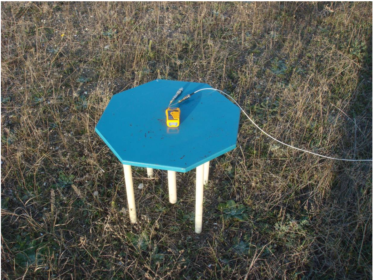
Fig. 11.8 — General view of test site for navigation test, point 2 (Configuration 8 - Beacon above ground plane).
