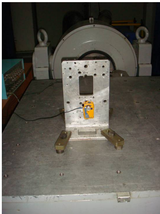
Figure 5.3 - General view of the horizontal axis X vibration test
