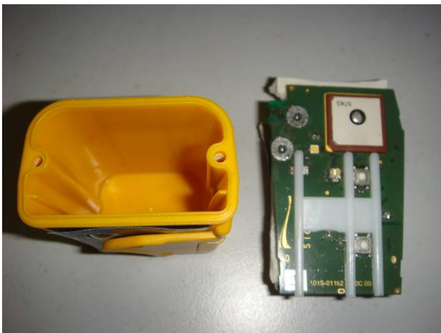
Figure 9.3 – View of the interiors of the Beacon upon completion of the Immersion Test. There is no water inside
