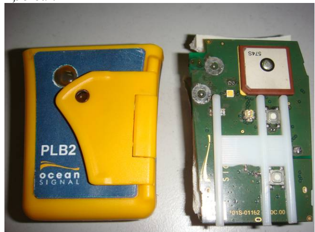
Figure 9.3 – View of the interiors of the Beacon upon completion of the Immersion Test. There is no water inside
