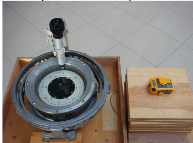
Figure 18.4 - The safety distance from EUT, after normalizing in stand-by mode to standard compass is 0,27 m.
