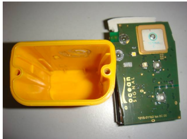
Figure 10.6 – View of the interiors of the Beacon upon completion of the Immersion Test. There is no water inside
