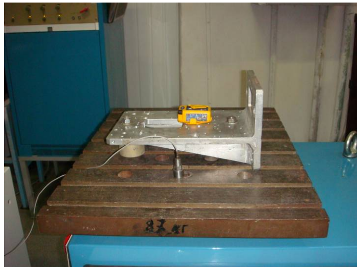
Figure 6.4 - Test Set-up. Lateral axis of the EUT. Longitudinal axis of the EUT
