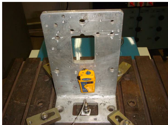
Figure 6.2 - Test Set-up. Vertical axis of the EUT
