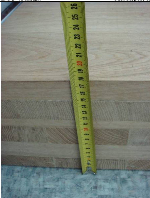
Figure 7.3 - Thickness of wood test surface
