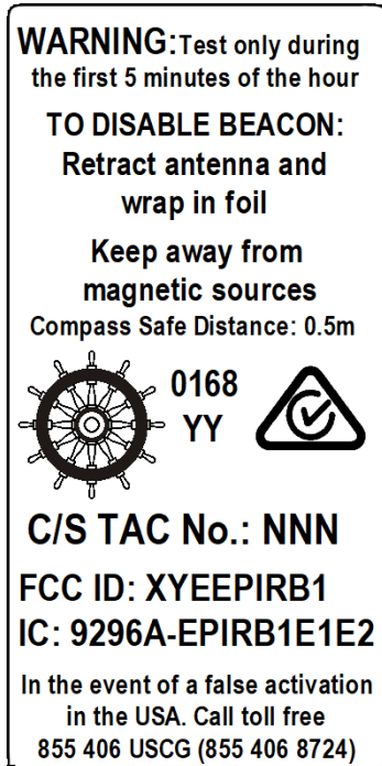
Figure 1: EPIRB1 Approvals Label showing FCC ID
