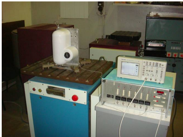
Figure 6.3 - Test Set-up. Vertical axis of the EUT with MRH
