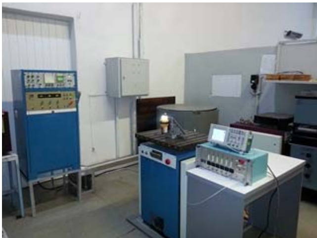
Figure 6.2 - Test Set-up. Vertical axis of the EUT with Manual bracket
