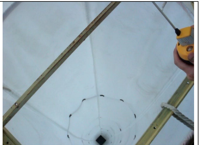
Figure 8.2 – Total view of test site of the drop test in water of EPIRB1 from a height of 20 m
