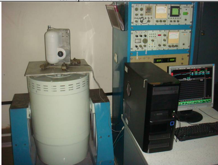
Figure 5.4 - General view of the test site vertical Z vibration (EPIRB1 with MRH)
