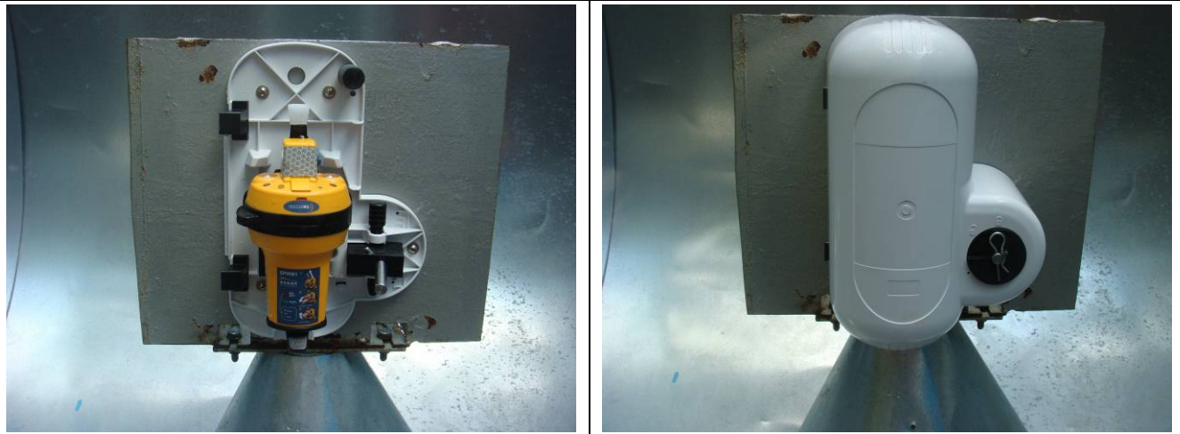
Figure 13.4 – EUT (EPIRB1 in MRH) mounted on the rotatable support before test.
