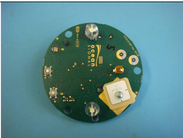
Figure 9.2 – The PCB (back view) after leakage and immersion tests. There is no water ingress.
