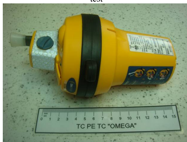
Figure 7.7 - View EUT upon completion of the drop test
