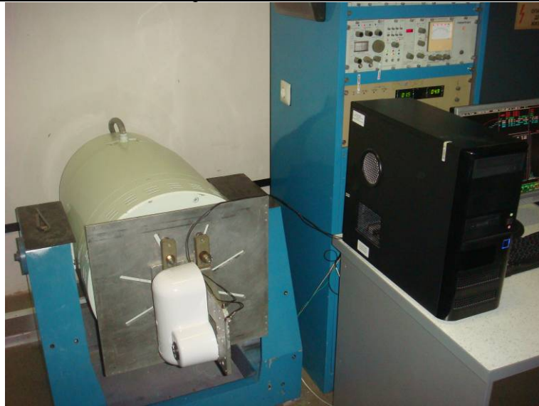
Figure 5.16 - General view of the horizontal Y vibration test (EPIRB1 with MRH)
