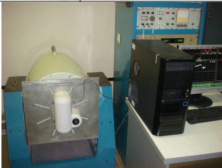
Figure 5.10 - General view of the horizontal X vibration test (EPIRB1 with MRH)
