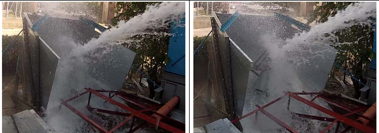
Figure 13.4 - The water washes EUT in an arc of 180°.
