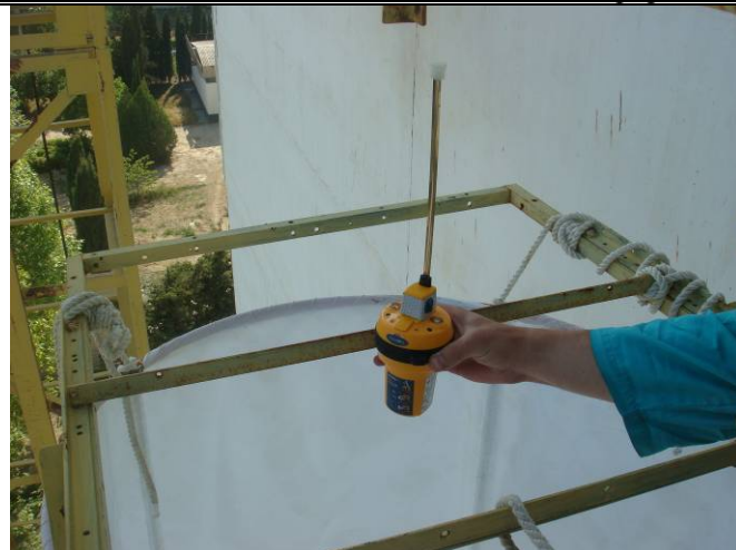
Figure 8.4 – View EPIRB1 dropping in water with antenna vertical up
