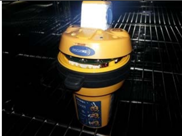
Figure 19.1 - View of the EPIRB with the opened housing before the humidity test
