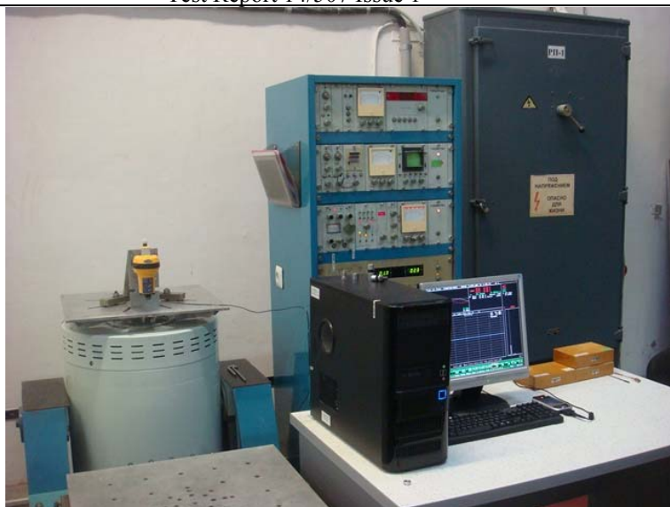
Figure 5.1 - General view of the test site vertical Z vibration (EPIRB1 with Manual Bracket)
