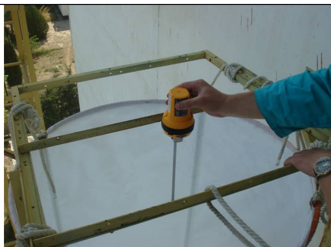
Figure 8.5 – View EPIRB1 dropping in water with antenna vertical down
