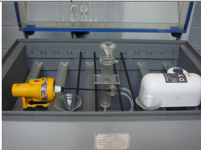
Figure 6.4 - View of the EUT (EPIRB) in salt fog chamber
