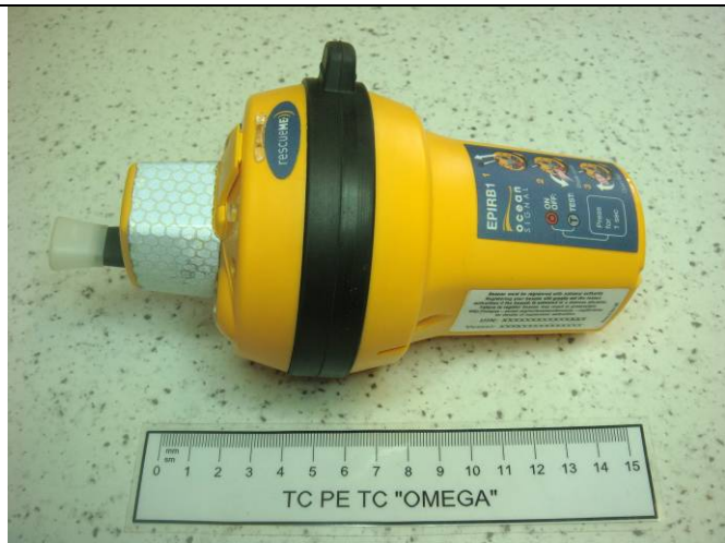
Figure 8.1 – View EPIRB1 before of the drop test in water
