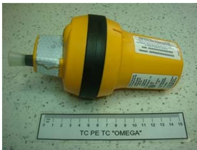
Figure 6.4 – View of the EUT upon completion of the Bump Test
