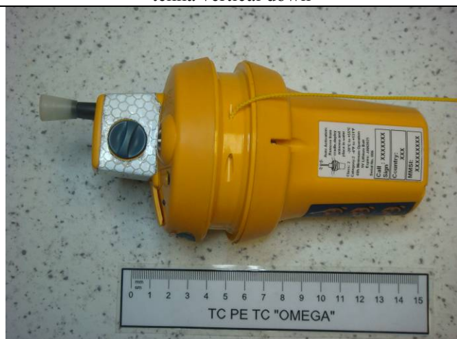
Figure 8.6 – Detailed examination of EPIRB1 upon completion of the drop test. There is no water inside.
