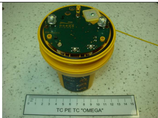
Figure 8.7 – Detailed examination of EPIRB1 upon completion of the drop test. There is no water inside.
