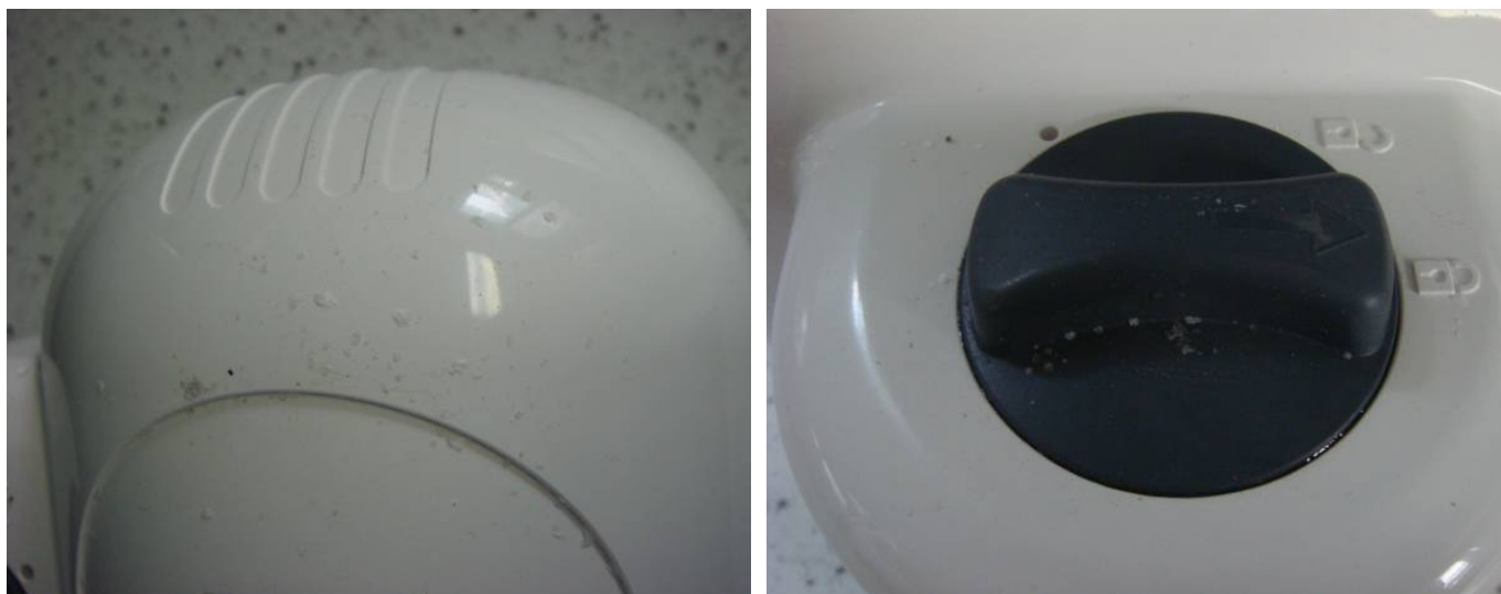
Figure 6.8 – View exterior inspection of EUT (EPIRB) upon completion the salt fog test
