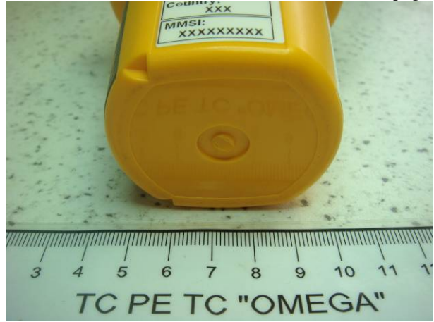
Figure 7.9 - View EUT upon completion of the drop test
