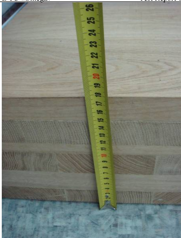
Figure 7.2 - Thickness of wood test surface
