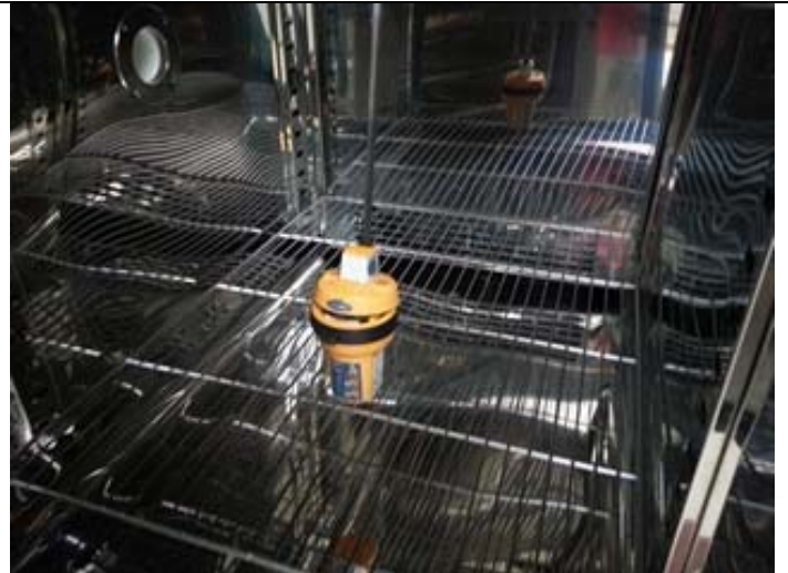
Figure 19.2 - View of the modified EPIRB installed in climatic chamber
