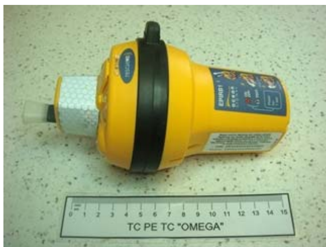
Figure 6.3 – View of the EUT upon completion of the Bump Test
