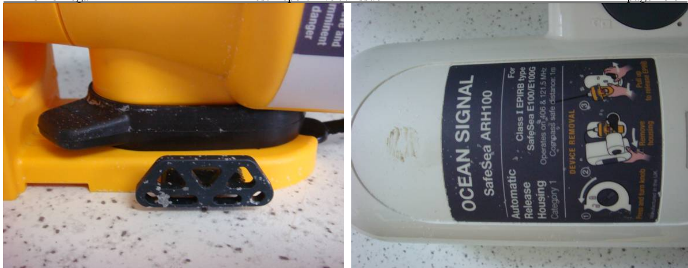
Figure 6.7 - View exterior inspection of EUT (EPIRB) upon completion of the salt fog test
