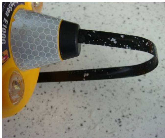
Figure 6.6 - View exterior inspection of EUT (EPIRB) upon completion of the salt fog test
