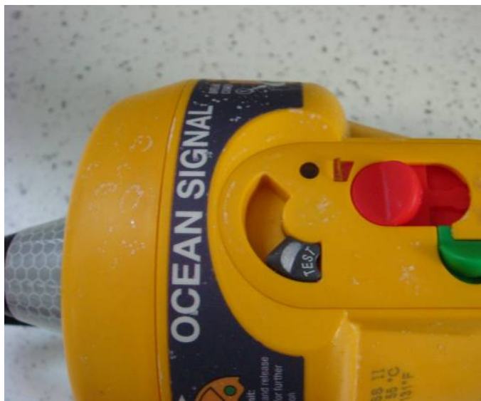
Figure 6.6 - View exterior inspection of EUT (EPIRB) upon completion of the salt fog test
