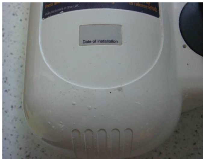
Figure 6.5 - View exterior inspection of EUT (EPIRB) upon completion of the salt fog test
