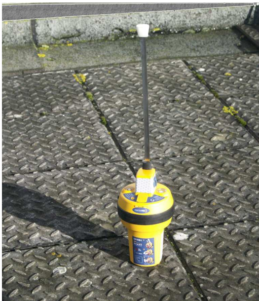
Figure 2: EPIRB1 Series Operating Mode – On Deck
