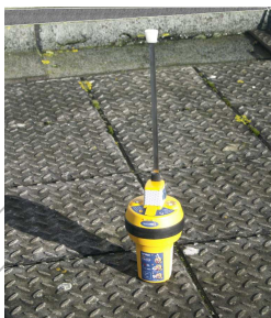
b) EPIRB deployed on deck
