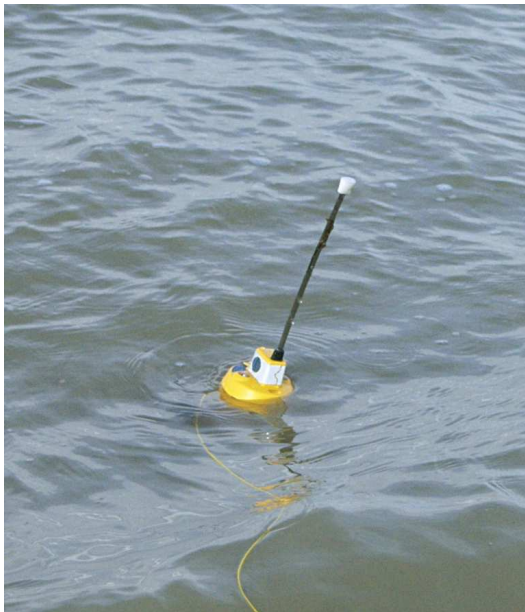
Figure 1: EPIRB1 Series operating Mode – Floating in water
