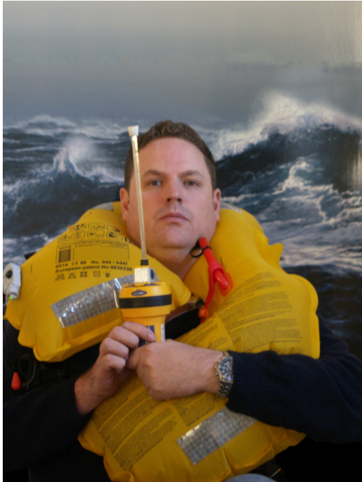
Figure 3: EPIRB1 Series Operating Mode – Handheld (representative of operation in a liferaft)
