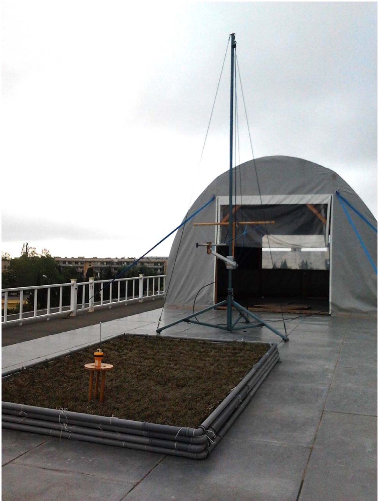
Fig 5.11.9 — General view of antenna test place at configuration 4 (section 4.5 C/S T.007), i.e. beacon operating above ground plane
