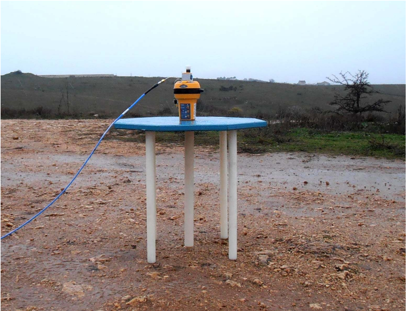
Fig. 5.11.2 — General view of test site for navigation test, point 2 (Configuration 8 - Beacon above ground plane).
