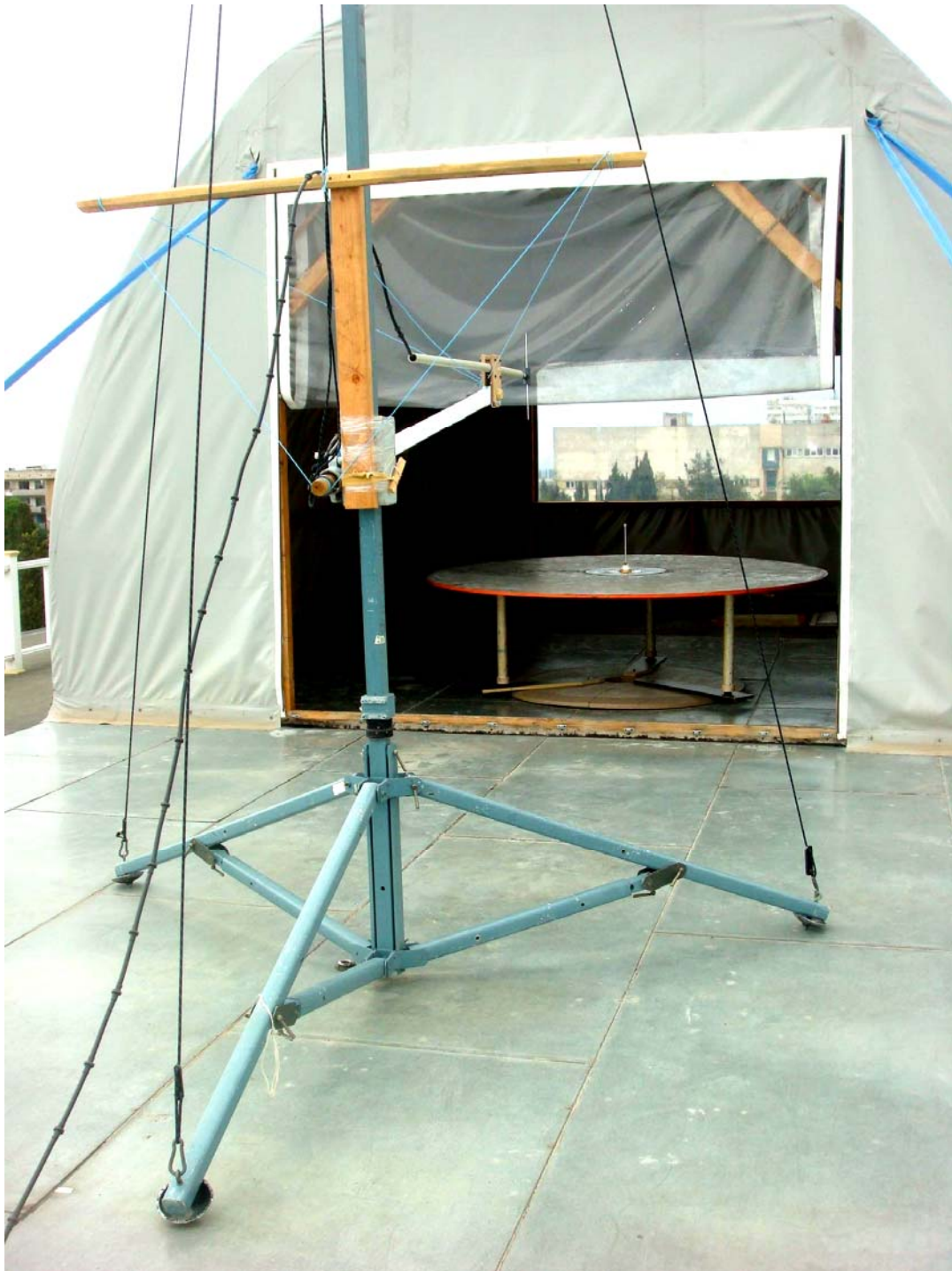
Fig 5.11.8 — General view of antenna test place at configuration 1 (section 4.5 C/S T.007), i.e. beacon “water” ground plane.
