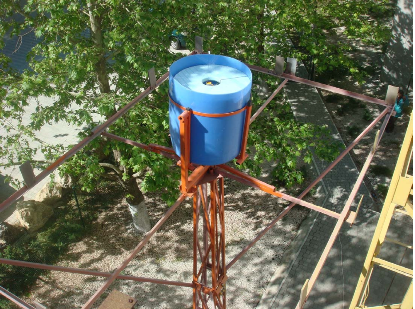
Fig 5.11.6 — General view of satellite qualitative test place at configuration 5 before rise up (section 4.5 C/S T.007), i.e. beacon operating while floating in the salt water. Beacon was raised above building
