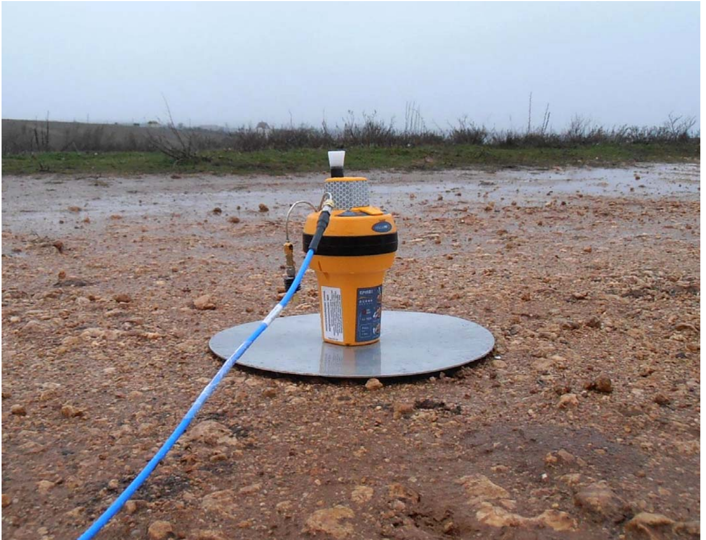
Fig. 5.11.1 — General view of test site for navigation test, point 2 (Configuration 7 – Beacon on ground plan).
