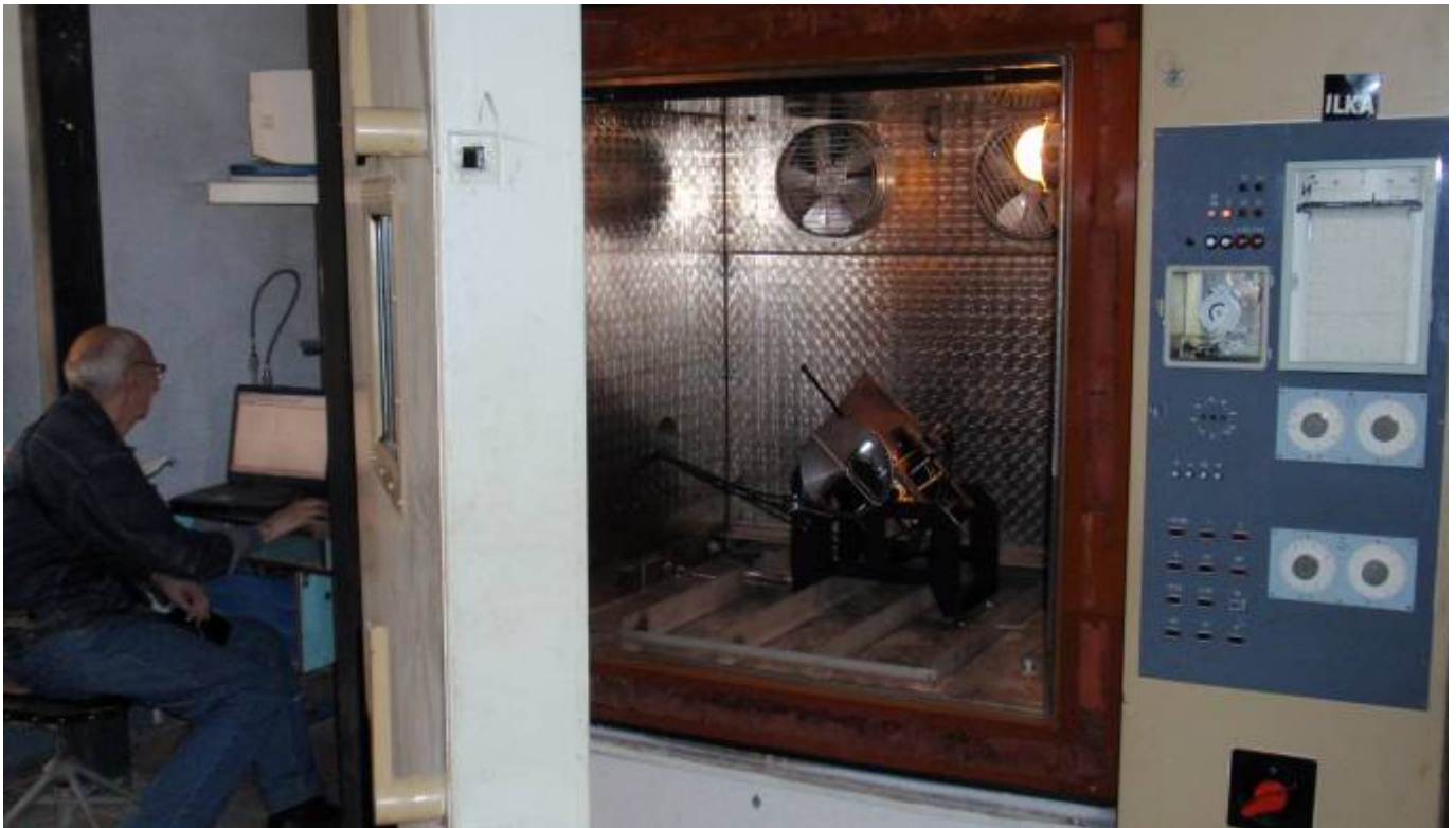
Figure 13.1 - Total view of equipment for strobe light test
