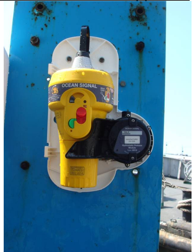
Figure 17.10 - View of the EUT (EPIRB and its release mechanism) upon completion inadvertent activation test
