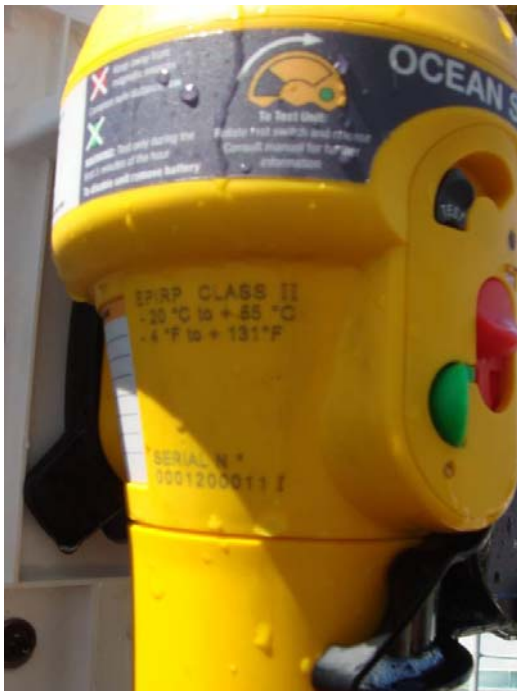
Figure 17.10 - View of the EUT (EPIRB and its release mechanism) upon completion inadvertent activation test
