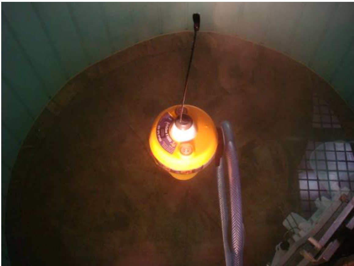
Figure 15.20 - View of automatic release mechanism in performance Upside down position after releasing and EPIRB activation
