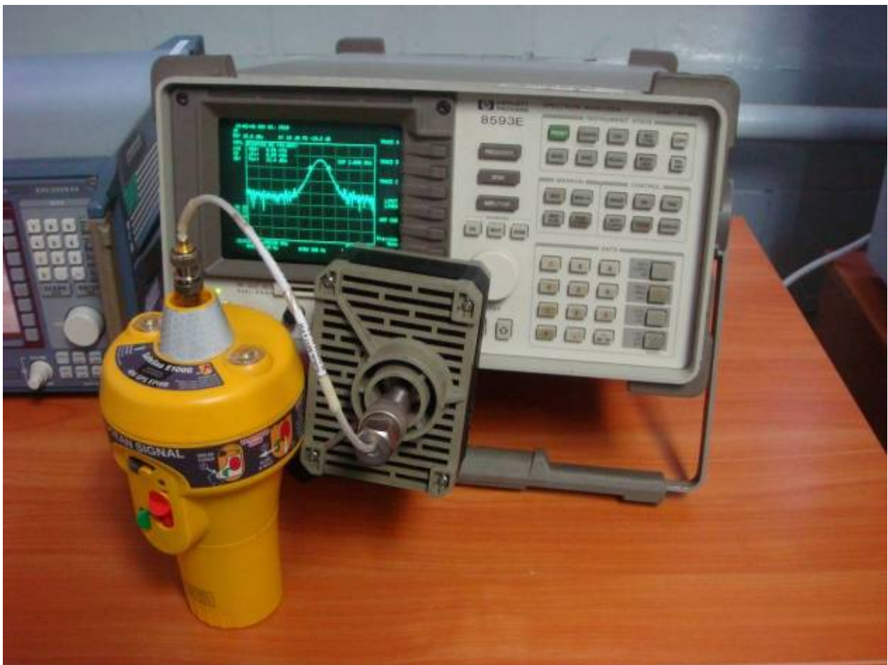
Figure 18.21 – Site for Carrier Frequency Test at the ambient temperature
