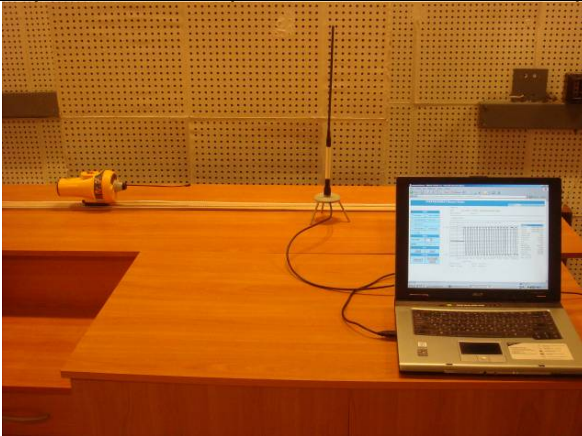
Figure 20.2 – View of the EUT (EPIRB E100G class 2) in a horizontal position.
