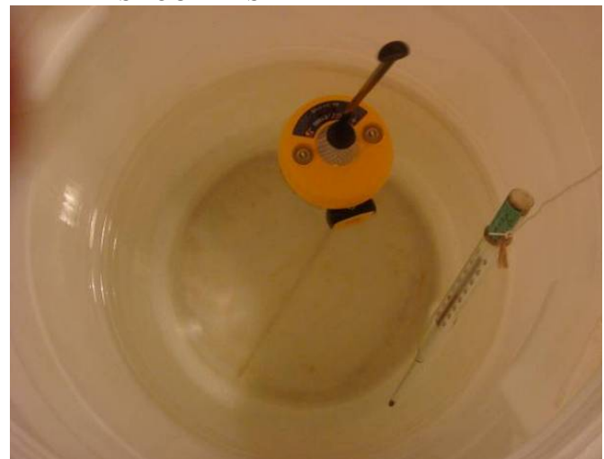
Figure 11.4 – View floated EUT (EPIRB) in fresh water
