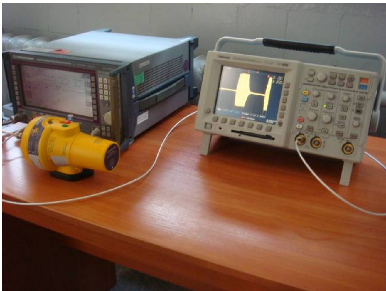
Figure 18.26 – Site for Modulation Characteristic Measurement at the ambient temperature
