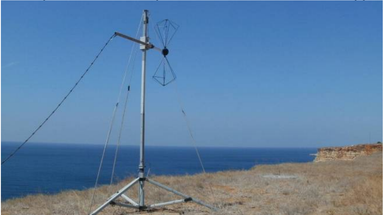
Figure 18.54 – Site for Peak Effective Radiated Power Measurement
