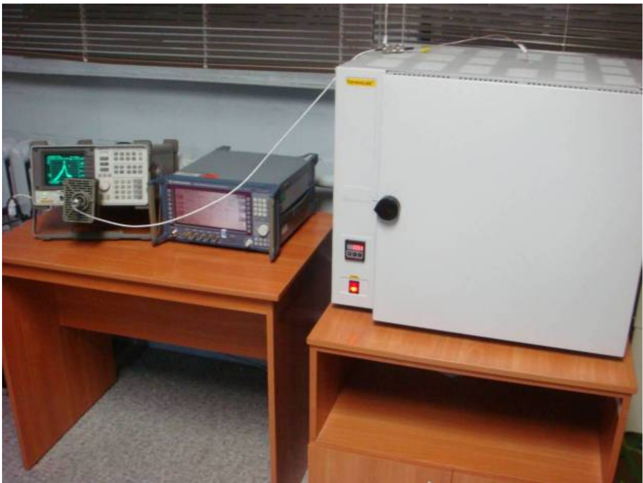
Figure 18.38 – Site for Carrier Frequency Test at the maximum operating temperature
