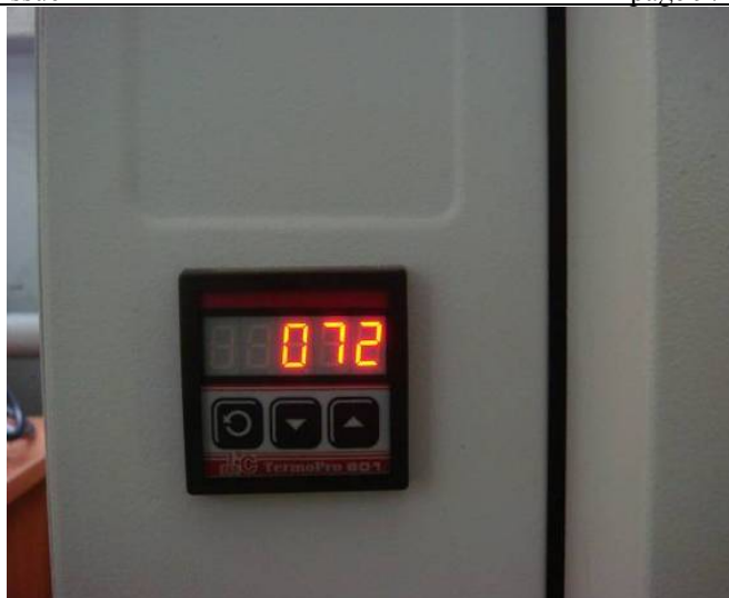
Figure 11.13 - View of maximum temperature soaking of EUT (EPIRB) in chamber before immersion in salt water.
