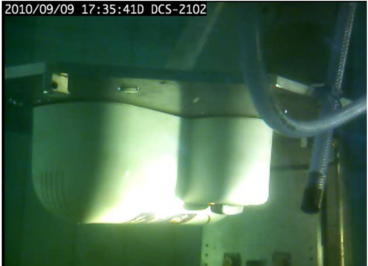
Figure 15.14 - View of mounting automatic release mechanism immersed into water in Rolling 90° bow down position before activation test
