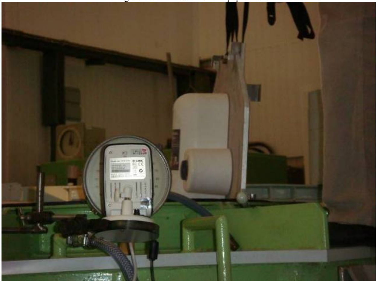
Figure 15.2 - View of mounting automatic release mechanism in performance position before activation test
