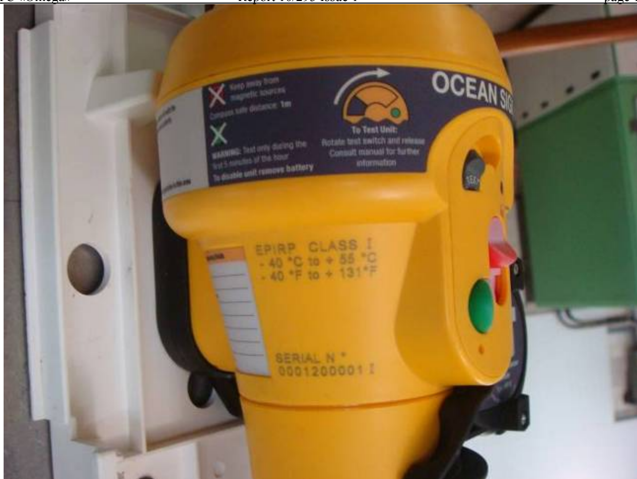
Figure 15.3 - View of EPIRB in mounting automatic release mechanism in performance position before activation test for EPIRB class 1
