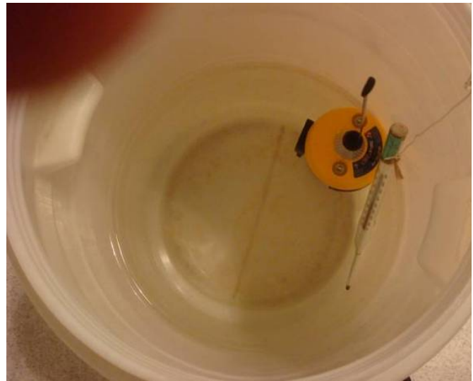
Figure 11.11 – View floated EUT (EPIRB) in fresh water.
