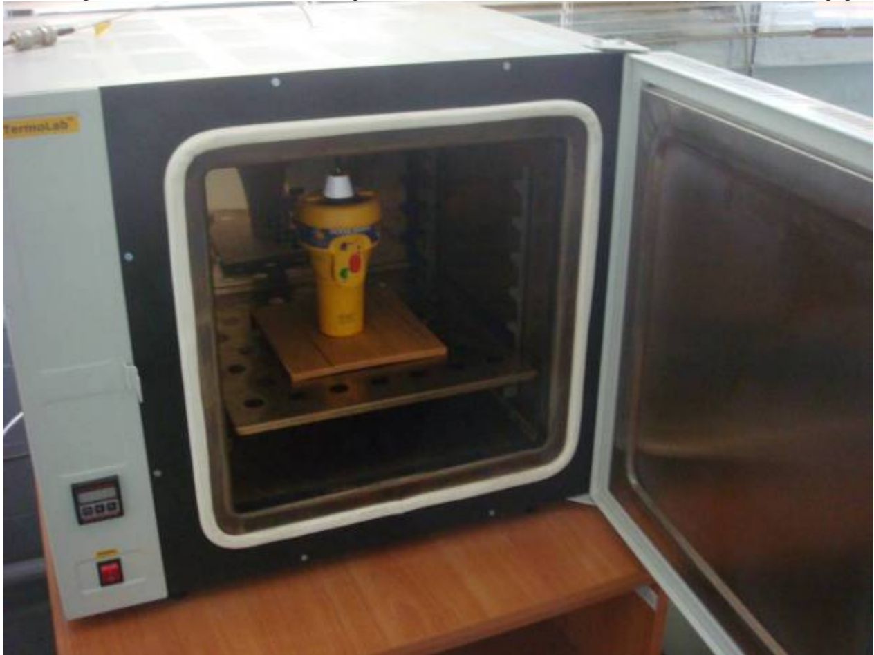
Figure 18.37 – Site for EUT (EPIRB) before Test at the maximum operating temperature
