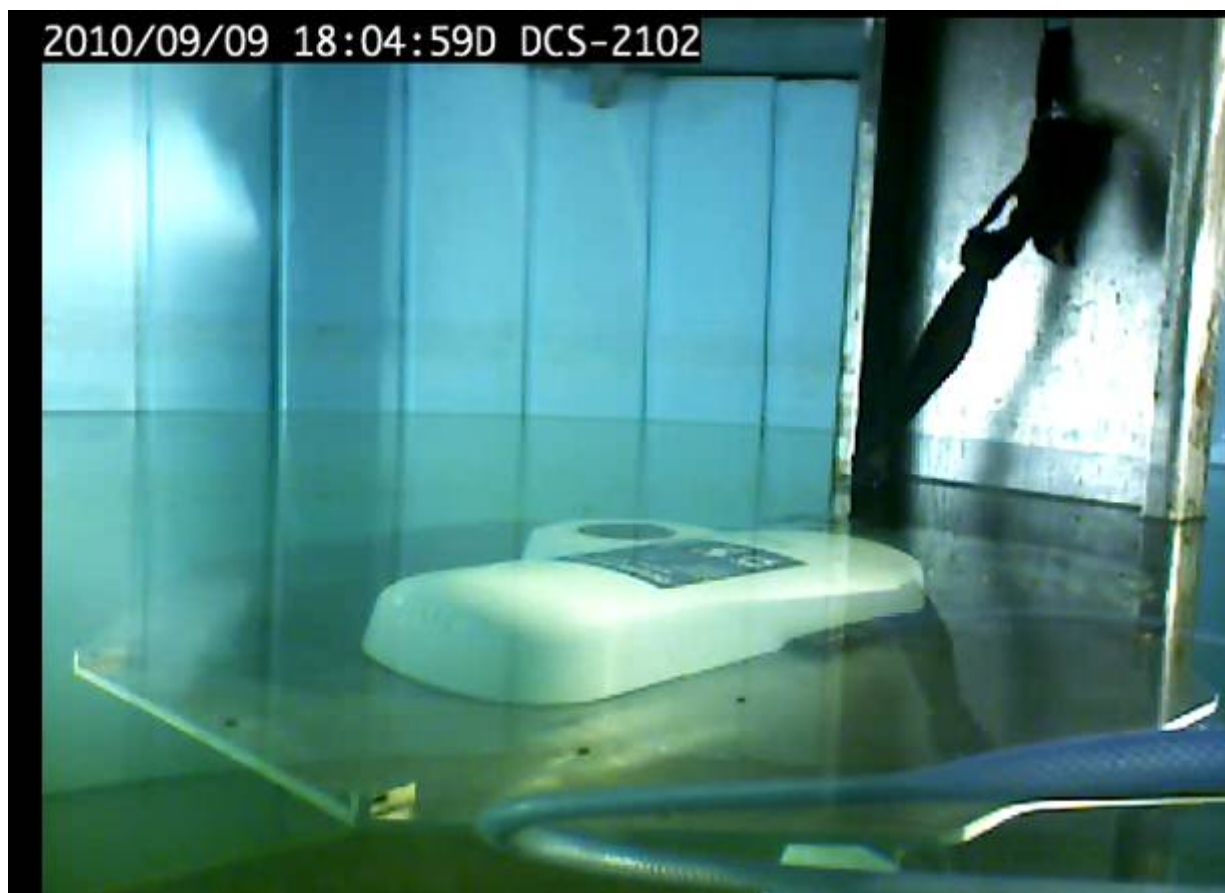
Figure 15.16– View of mounting automatic release mechanism immersed into water in Rolling 90° stern down position before activation test
