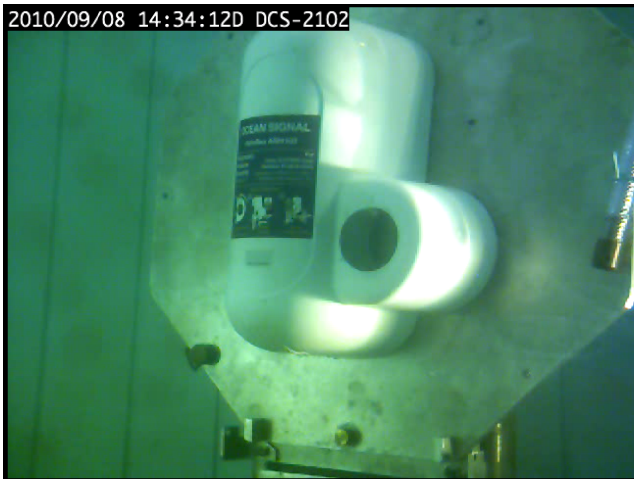
Figure 15.23 – View of mounting automatic release mechanism class 2 immersed into water in performance position before activation test
