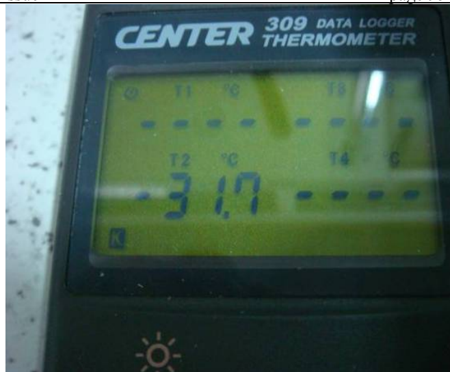
Figure 11.6 - View of minimum temperature soaking of EUT (EPIRB) in chamber before immersion in salt water.
