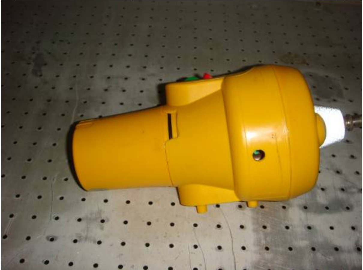
Figure 19.1 - View of the EUT (EPIRB E100G class 2) before the humidity test
