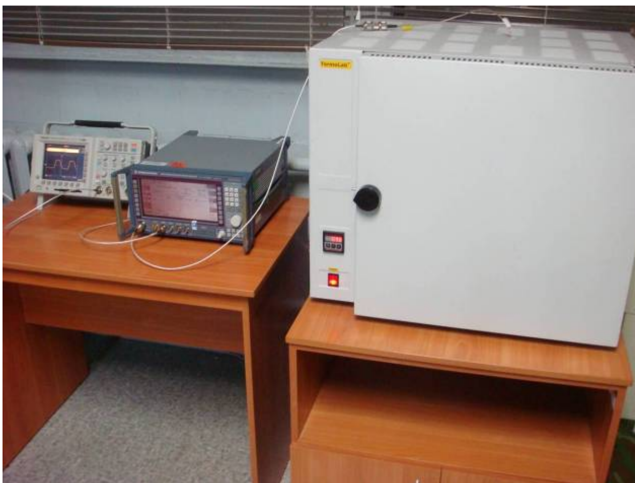
Figure 18.43 – Site for Modulation Characteristic Measurement at the maximum operating temperature
