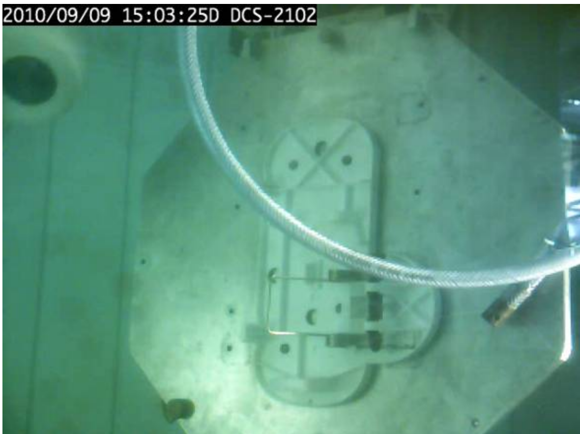
Figure 15.8 – View of automatic release mechanism in performance position at the moment of activation
