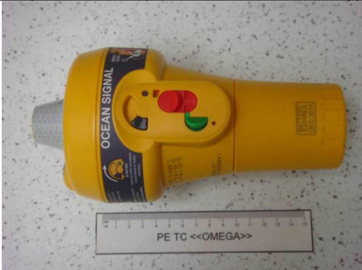
Figure 18.1 – View of the EUT (EPIRB) before the auxiliary radio-locating device transmitter test
