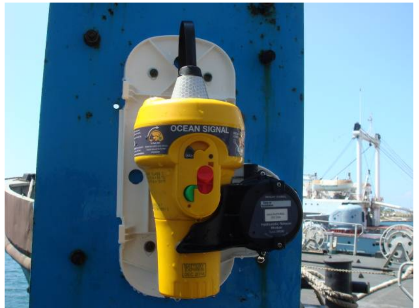
Figure 17.10 - View of the EUT (EPIRB and its release mechanism) upon completion inadvertent activation test
