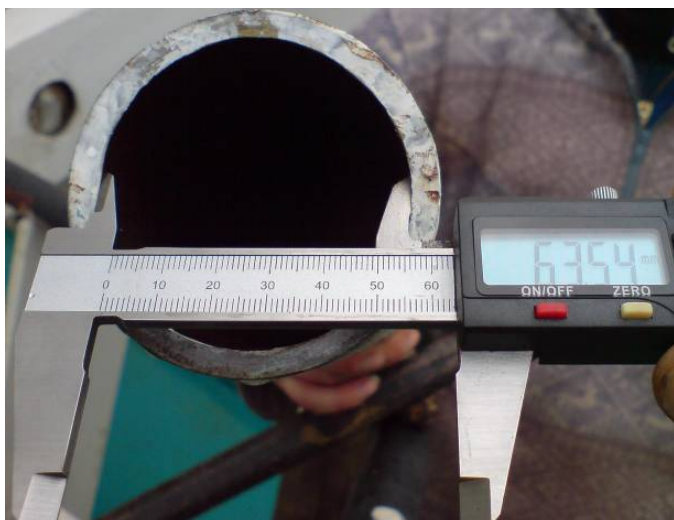
Figure 17.6 - View of the nozzle hose that has a diameter of 63.5 mm
