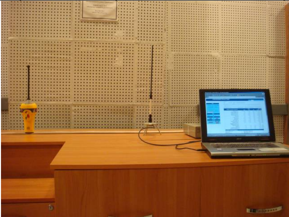
Figure 20.4 - View of the EUT (EPIRB E100G class 2) in a initial upright position
