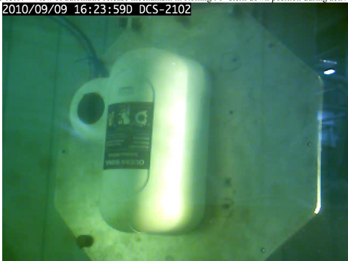
Figure 15.18 - View of mounting automatic release mechanism immersed into water in Upside down position before activation test
