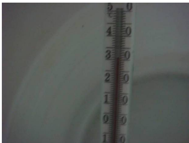
Figure 11.15– The temperature of salt water for EUT (EPIRB) immersion (+31 °C).
