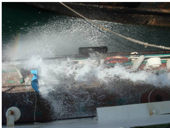
Figure 17.7 - View of EUT during the test. The water strike EUT straight
