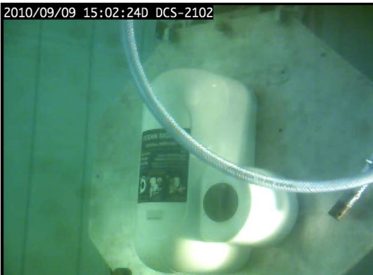
Figure 15.6 - View of mounting automatic release mechanism immersed into water in performance position before activation test
