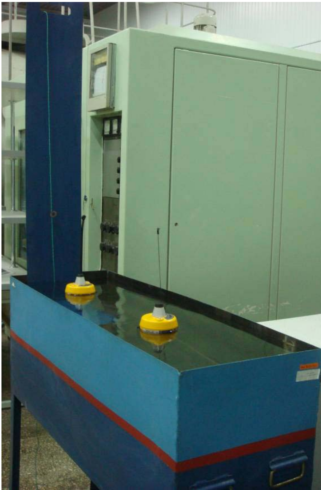
Figure 16.1 – View of the EUT (EPIRB) before the stability and buoyancy test
