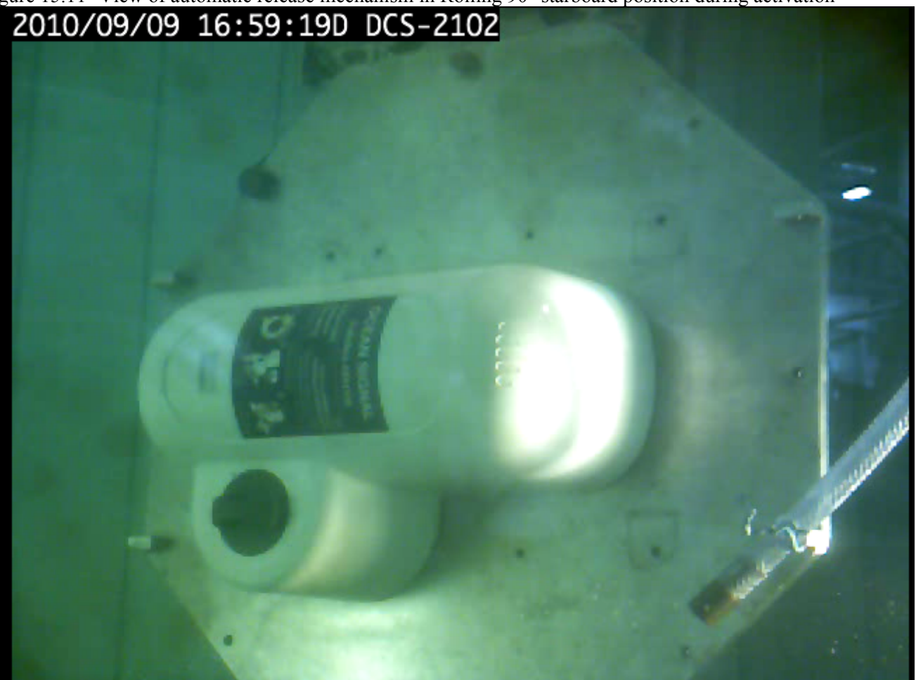
Figure 15.12 – View of mounting automatic release mechanism immersed into water in Rolling 90° port position before activation test
