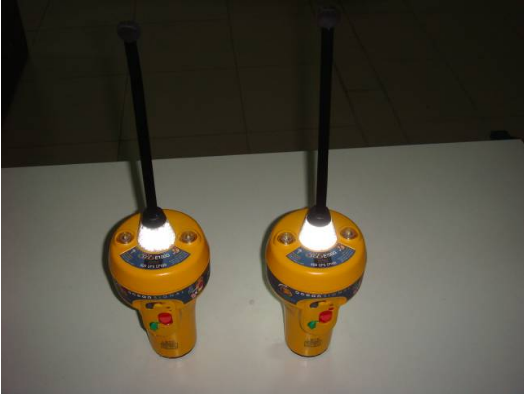
Figure 16.5 – View of the EUT (EPIRB) upon completion of the stability and buoyancy test
