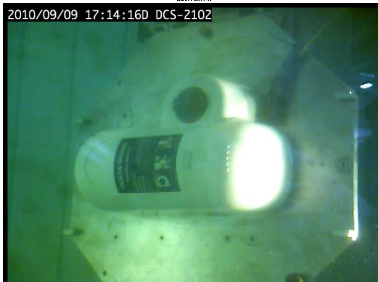
Figure 15.10 - View of mounting automatic release mechanism immersed into water in Rolling 90° starboard position before activation test
