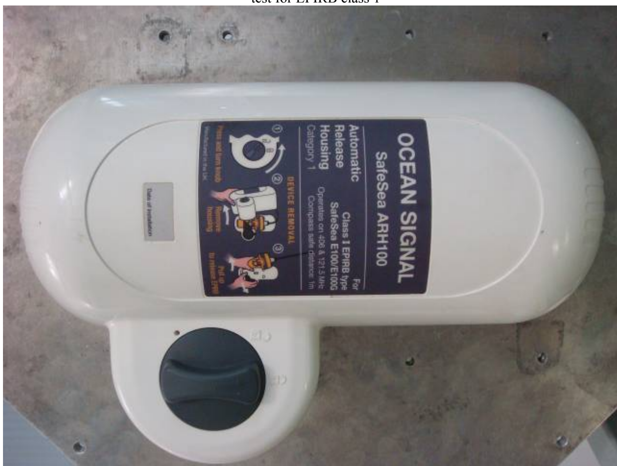
Figure 15.4 - View of mounting automatic release mechanism class 1 in performance position before activation test
