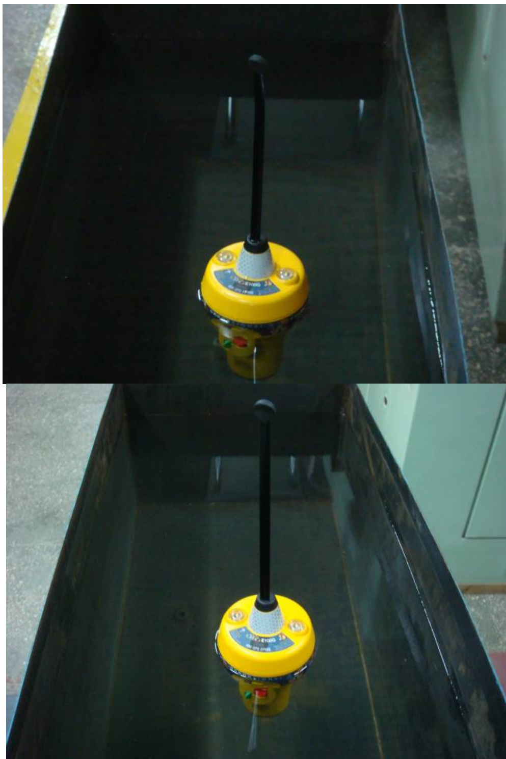
Figure 16.5 – The EUT (EPIRB) buoyancy test
