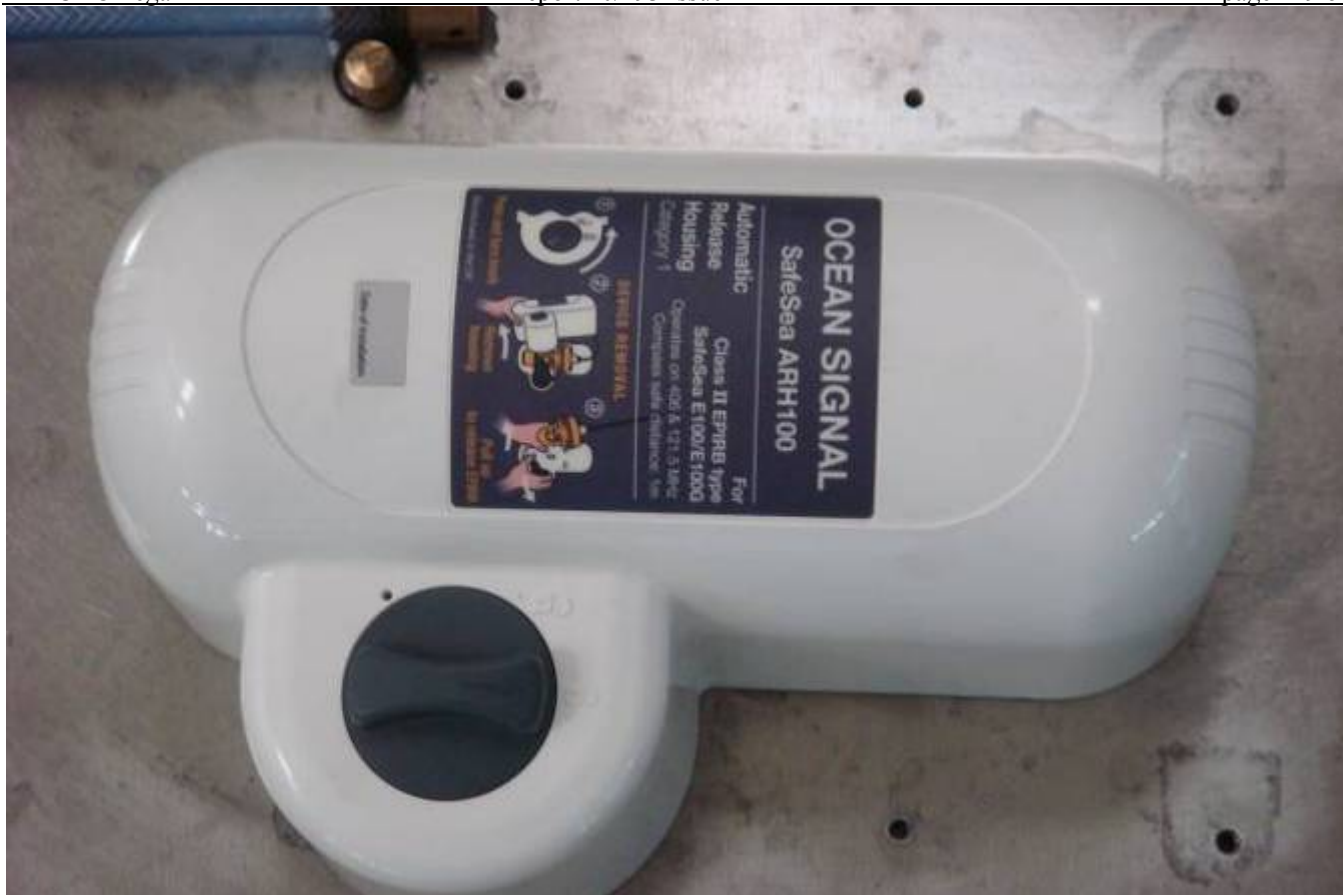
Figure 15.22 View of mounting automatic release mechanism class 2 in performance position before activation test
