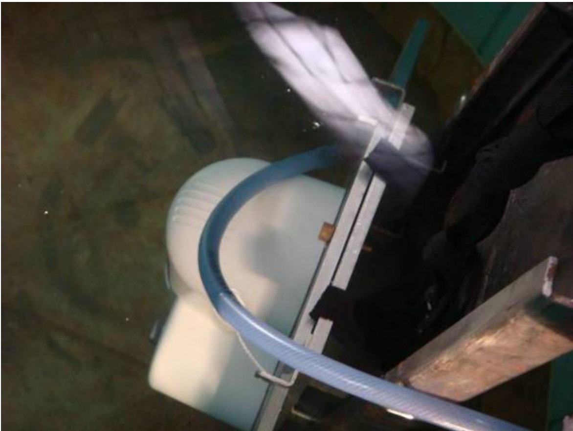
Figure 15.5 - View of mounting automatic release mechanism immersed into water in performance position before activation test
