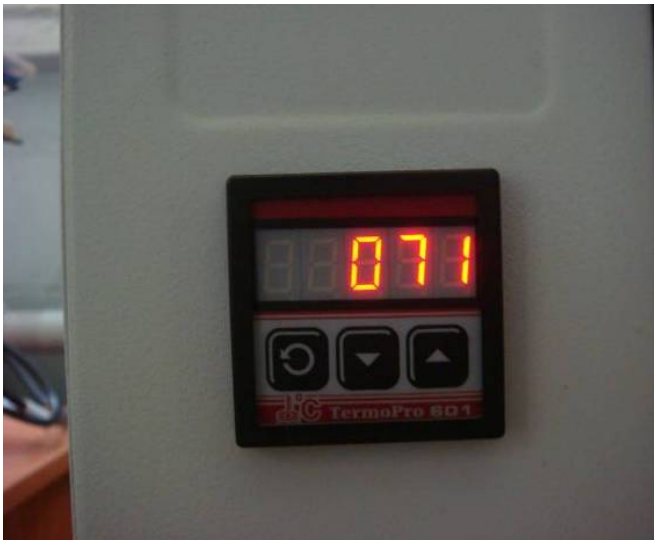
Figure 11.10 - View of maximum temperature soaking of EUT (EPIRB) in chamber before immersion in fresh water.
