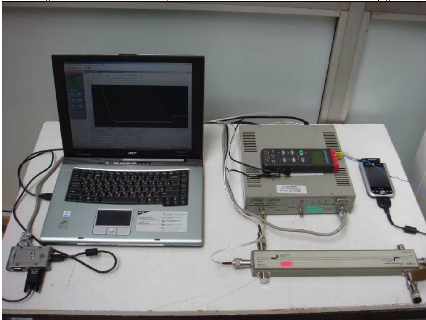
Figure 12.1 – View EUT (EPIRB SafeSea E100G class 2 ) before the OPERATIONAL LIFE TEST
