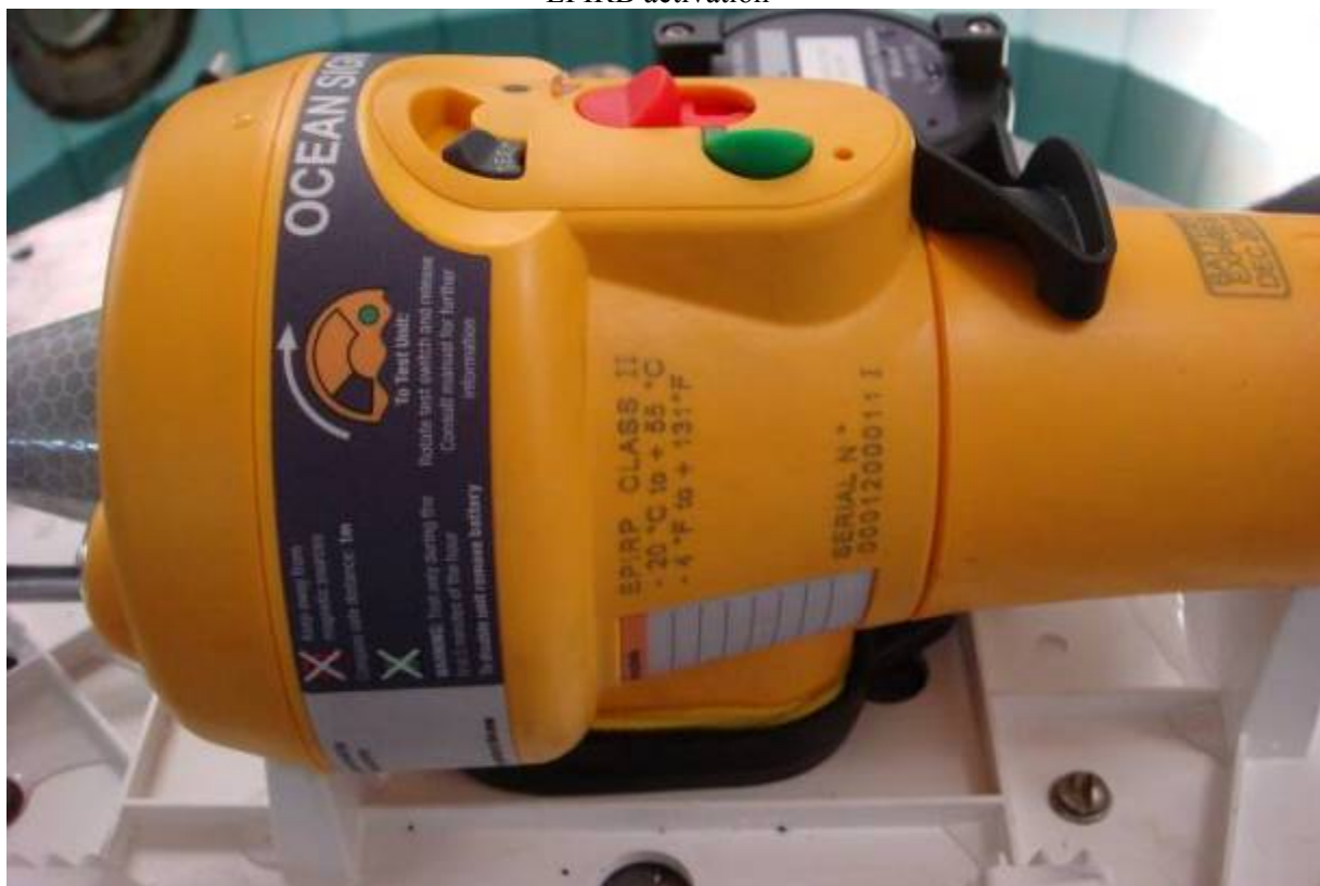
Figure 15.21 - View of EPIRB in mounting automatic release mechanism in performance position before activation test for EPIRB class 2
