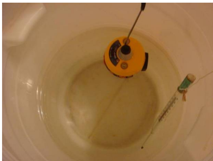
Figure 11.14 – View floated EUT (EPIRB) in salt water
