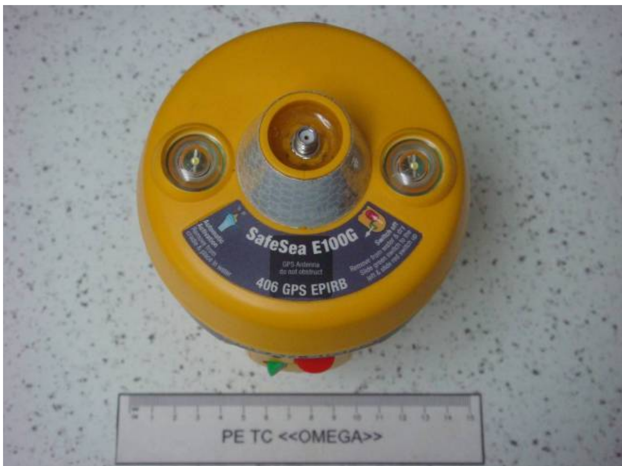
Figure 18.2 – View of the EUT (EPIRB) before the auxiliary radio-locating device transmitter test
