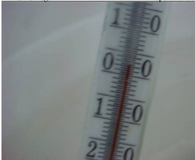
Figure 11.5 – The temperature of fresh water for EUT (EPIRB) immersion (+2.5 °C).
