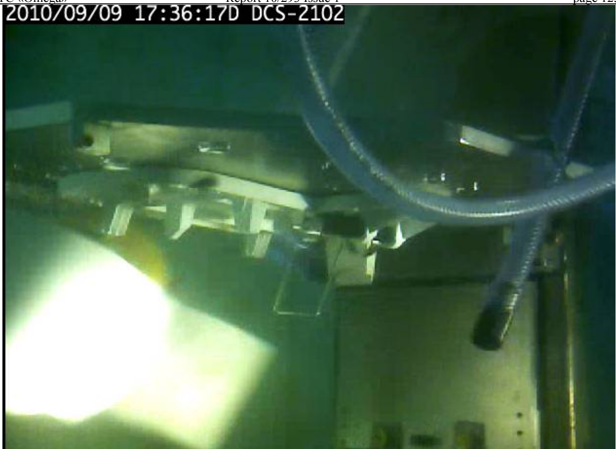
Figure 15.15 - View of automatic release mechanism in Rolling 90° bow down position during activation
