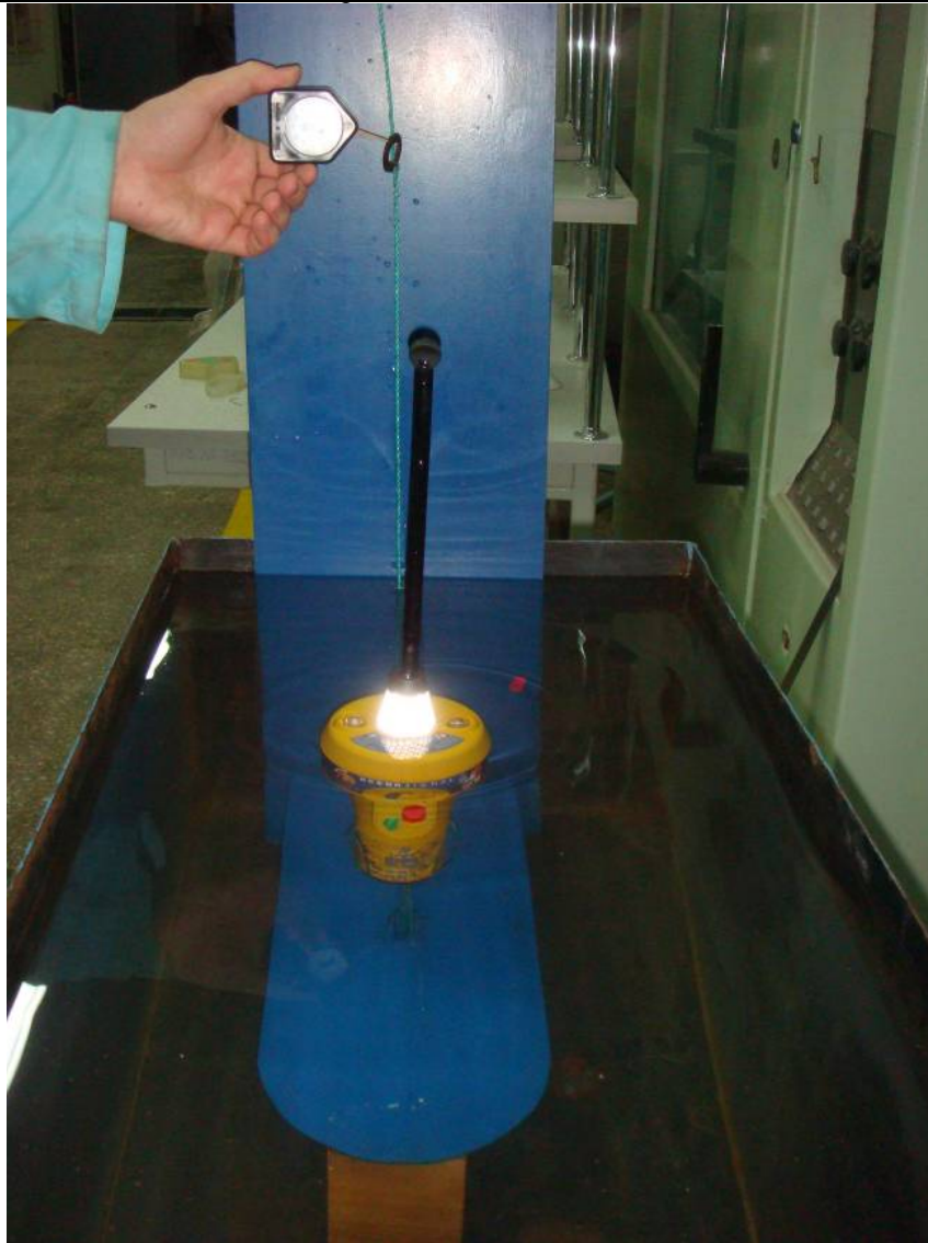
Figure 16.3 – The EUT (EPIRB) stability test
