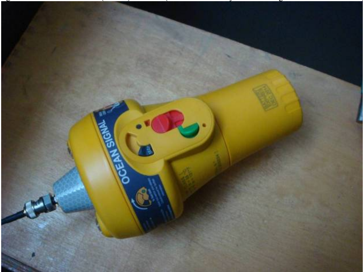
Figure 18.4 – Site for EUT (EPIRB) before Test at the minimum operating temperature
