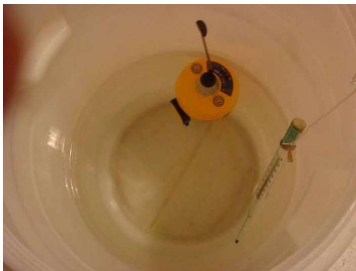
Figure 11.7 – View floated EUT (EPIRB) in salt water
