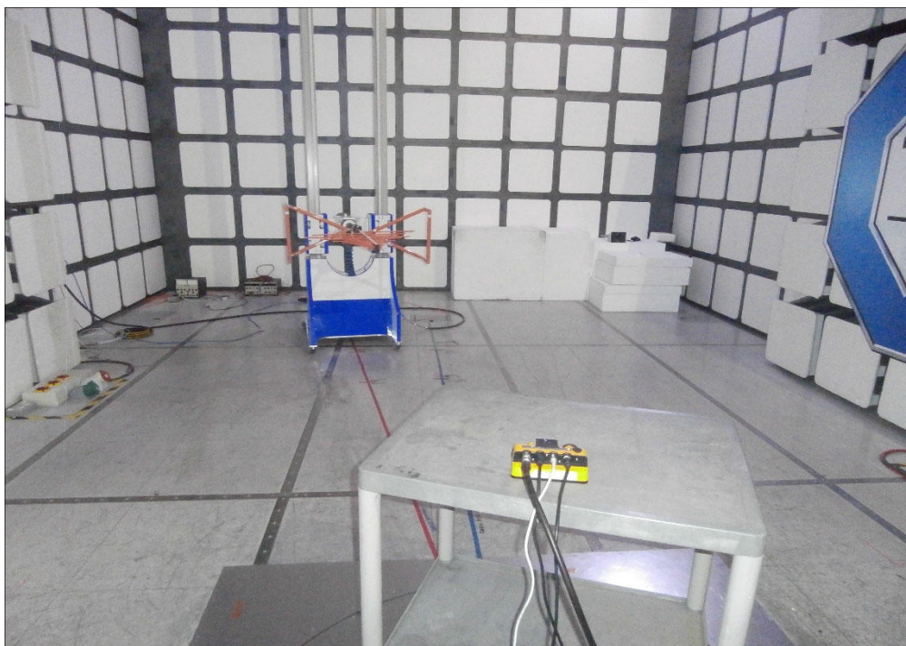
Figure 6 - Test Setup - Radiated Emissions 30 MHz to 1 GHz
