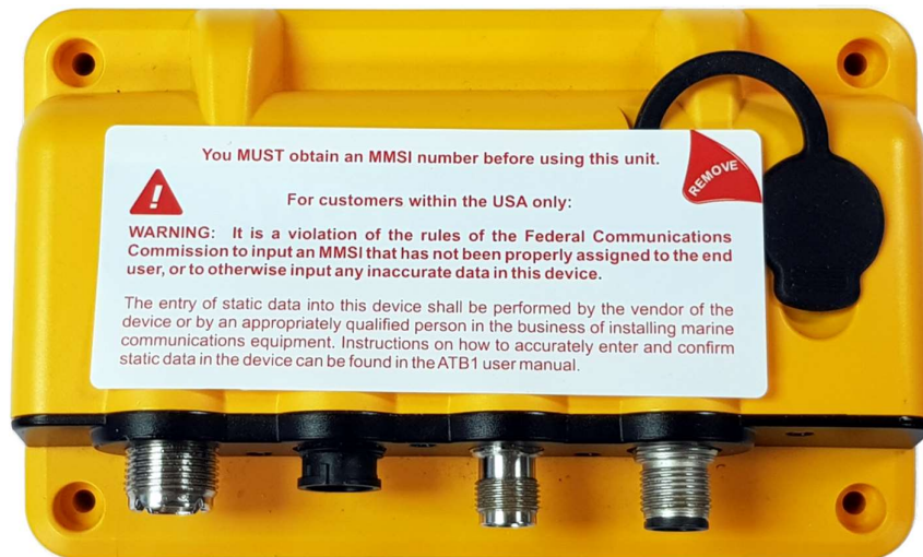
Figure 10: ATB1 with FCC MMSI warning label
