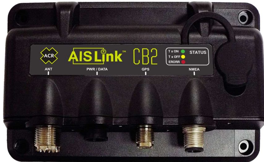
Figure 7: ACR AISLink CB2 OEM Variant – Top view showing labelling
