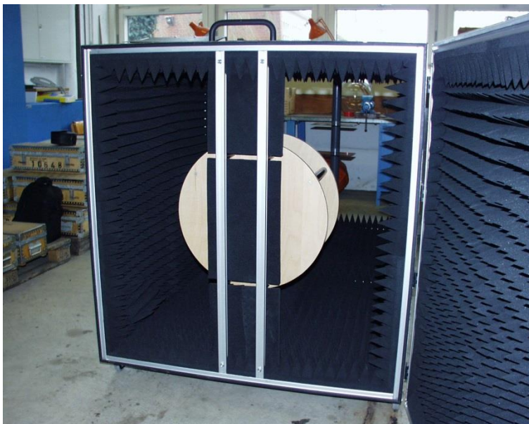
GPS test box, interior view
