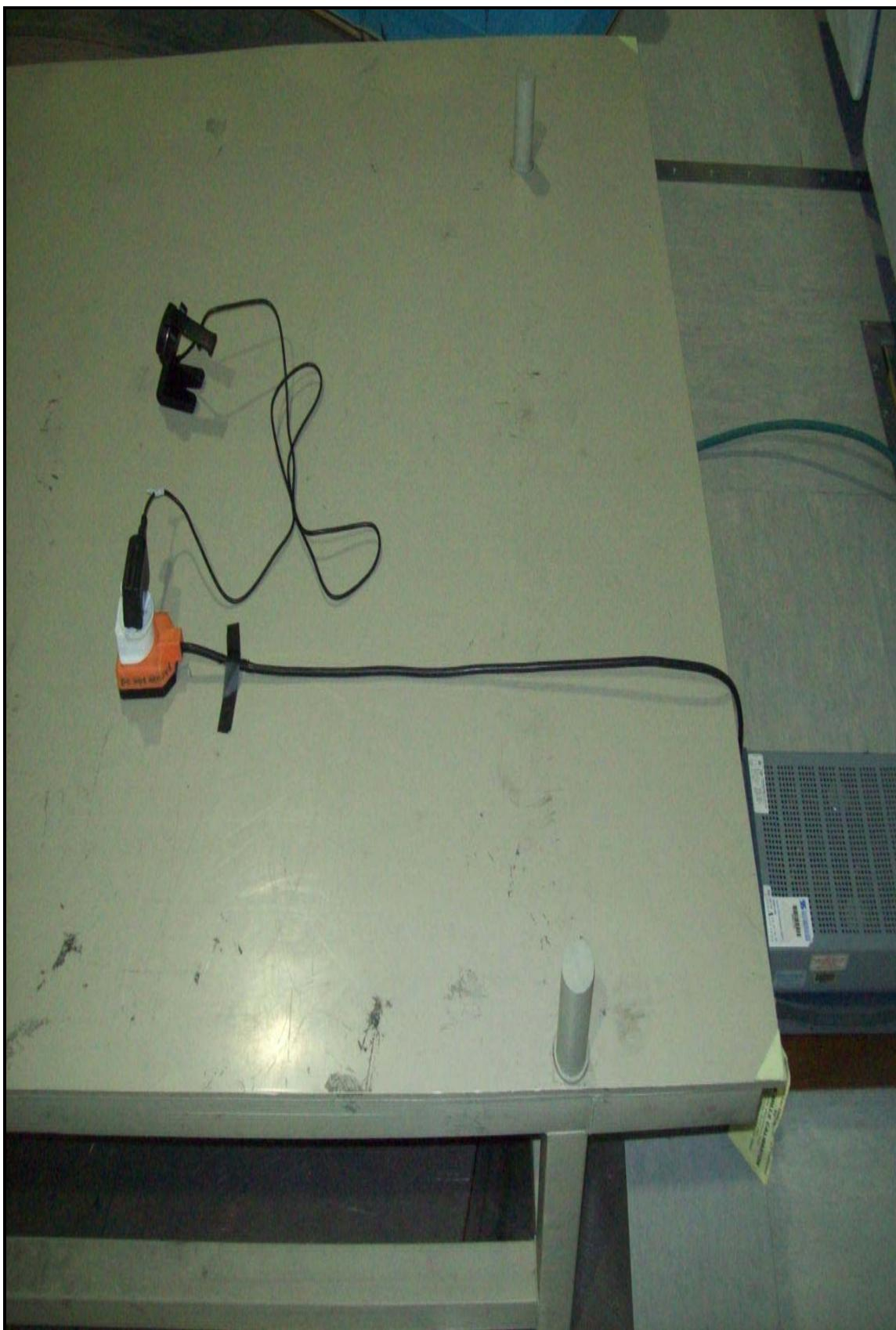
**PHT\79720JD01\002 - Test Configuration Photograph - Radiated Emissions**
