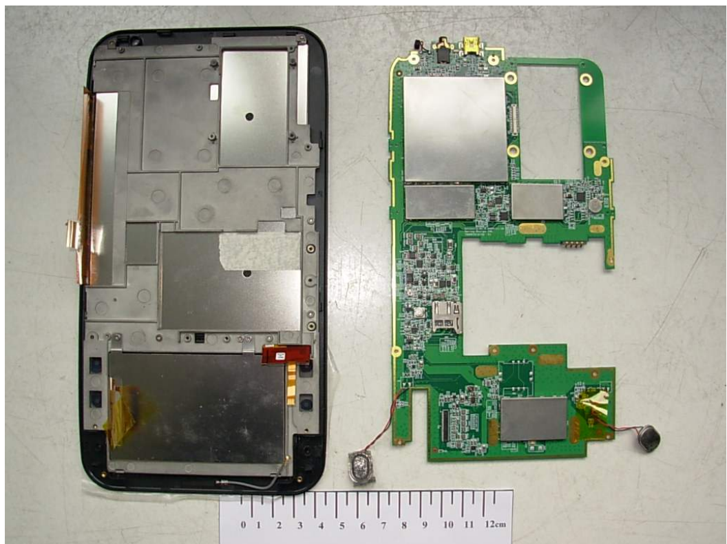
FIGURE 4 ALEX™ READER(M/N: DS-10) COVER REMOVED #2
