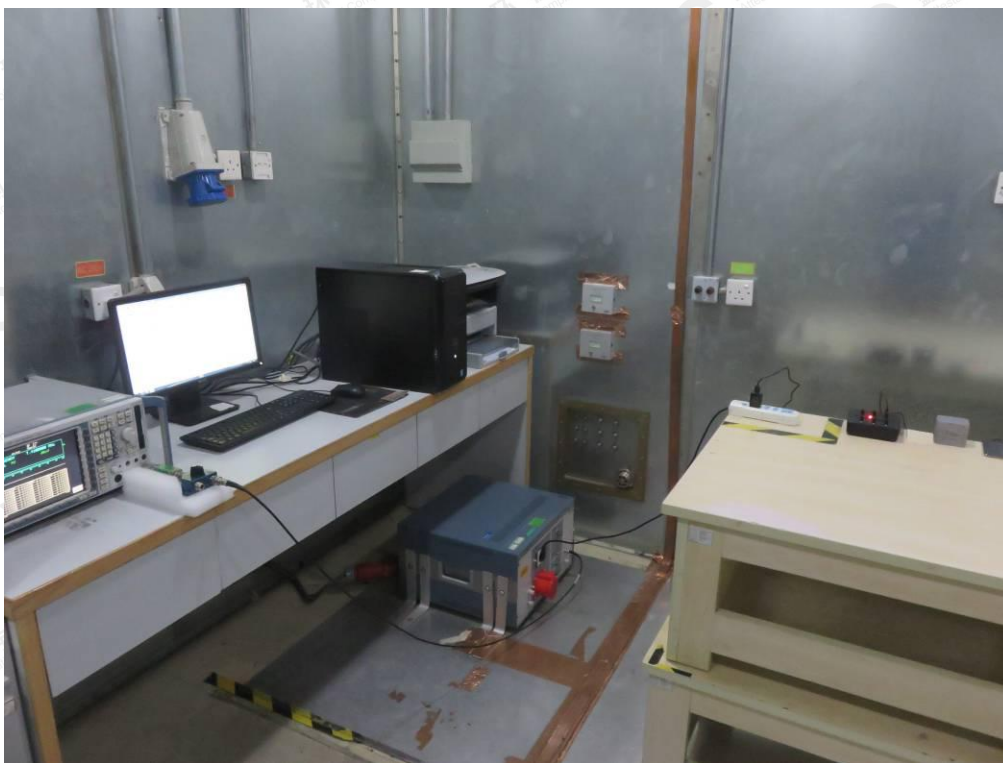
FCC RADIATED EMISSION TEST SETUP
